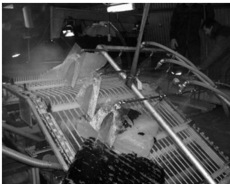
Fig. 6.17 Lifting Grated Belt (LGB) Oil Recovery Device with Flushing System (tested in HSVA's Arctic Environmental Test Basin)
