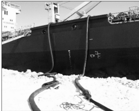
(← Fig. 6.4) Connection between end of pipeline to the manifolds of MT UIKKU
