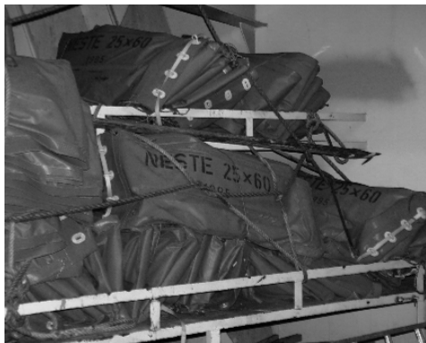
(← Fig. 6.13) Floating oil booms stored in the forecastle of MT UIKKU
