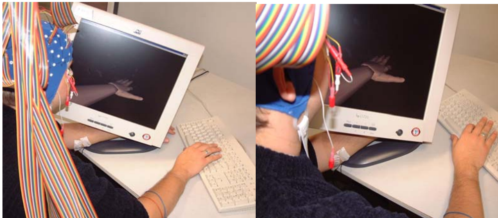
Figure 41: User and monitor position in experiments with the “Virtual Arm” feedback scenario. Monitor is placed and rotated such that the user’s imagination of observing the own arm while looking on the screen is maximized.
