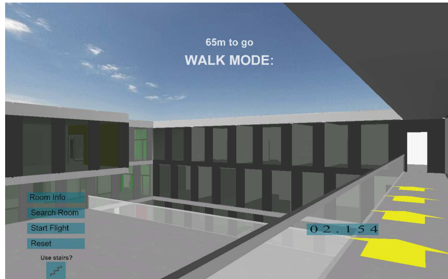
Figure 3.12: A snapshot of a VRML model for calculating the shortest path and guiding to the destination in the reference model (Computer Science building at the Universität Stuttgart)
