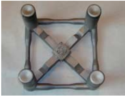
Fig. 7.1. Casting according to the German aeronautic standard (Later on - Casting 1)
