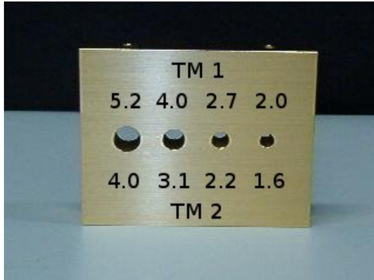
Figure 115: Golden plate with four different apertures. The numbers in top and bottom correspond to the aperture size in beam radii for TM 1 and TM 2, respectively.
