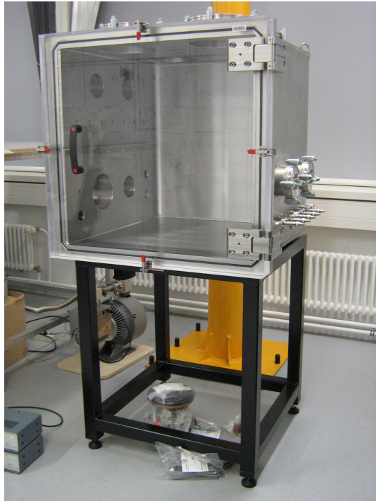
Figure 19: Photograph of the vacuum chamber for the PAAM test facility.
