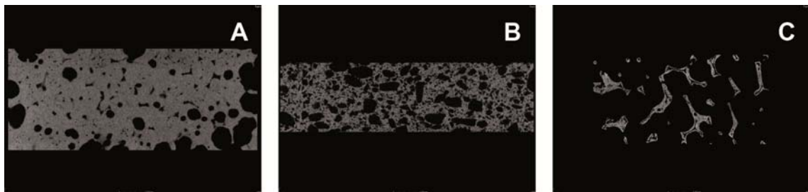
Fig. 2.11: Vertical cross-section of Osseolive, sample 2 with 12.8 % porosity (A), Cerasorb M (B) and 45S5-Bioglass (B), generated by a nanoCT scan.
