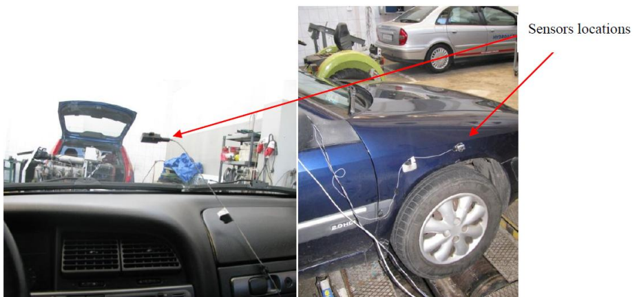
Fig. 4. Sensors sixinf for measuring: on the glass (a) and car body, above the wheel (b)
