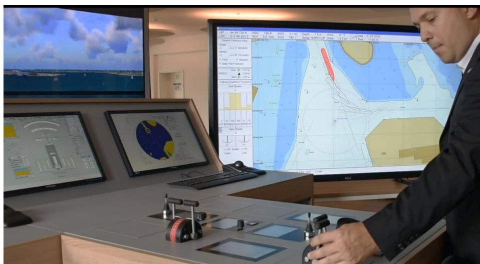
Fig. 5 Manoeuvring Monitoring & Conning Module – Demo of using bridge handles in to train "Touch and Feel" for Controls with Multiple Dynamic Prediction showing the effect of any control change immediately as future ship shape on ENC (SAMMON Demo on Bridge
