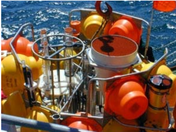
Fig. 5.5.3: Position of the two sediment traps (tripllett and cone).
