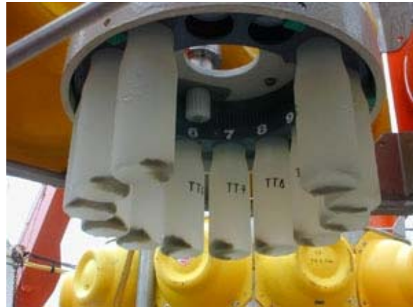
Fig. 5.5.4: View from below on the 12 bottles of the cone-shaped trap after recovery.
