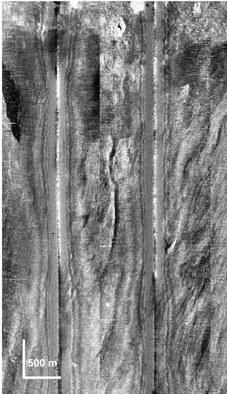
Fig. 5.1.10: Processed 75 kHz sidescan mosaic showing an area with intensive lineations on the northern flank of the southern summit of Hydate Ridge
