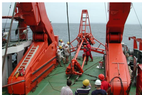
Figure 2. BGS Rockdrill during drilling operations with R/V Sonne at Conical Seamount (New Ireland fore-arc, PNG).
