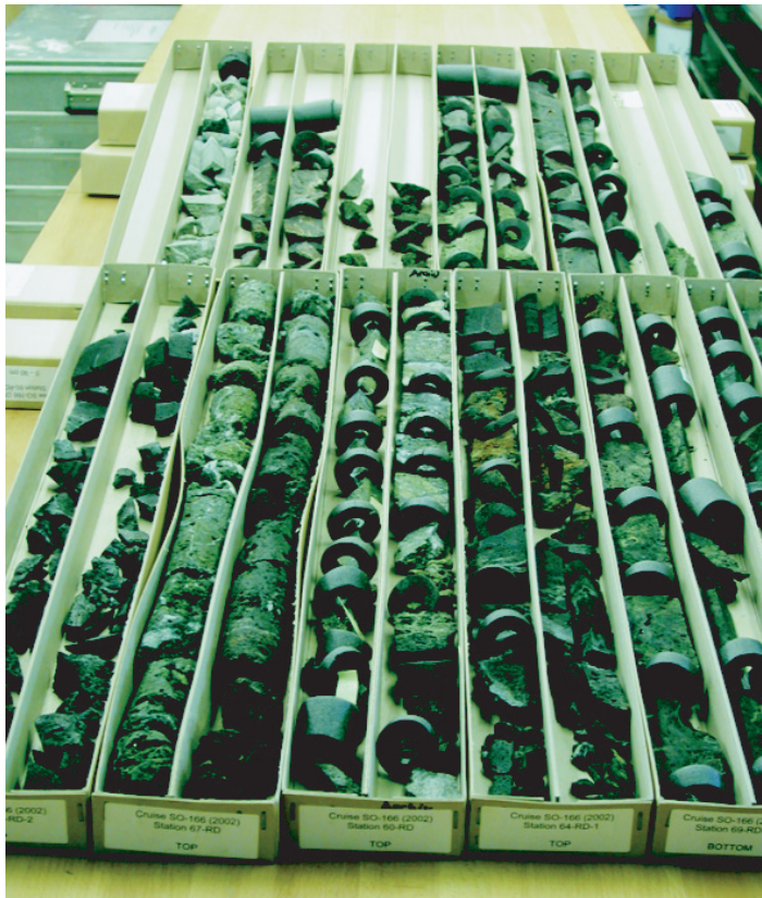
Figure 4. Drill core recovered with the BGS Rockdrill from the Pacmanus hydrothermal field.
