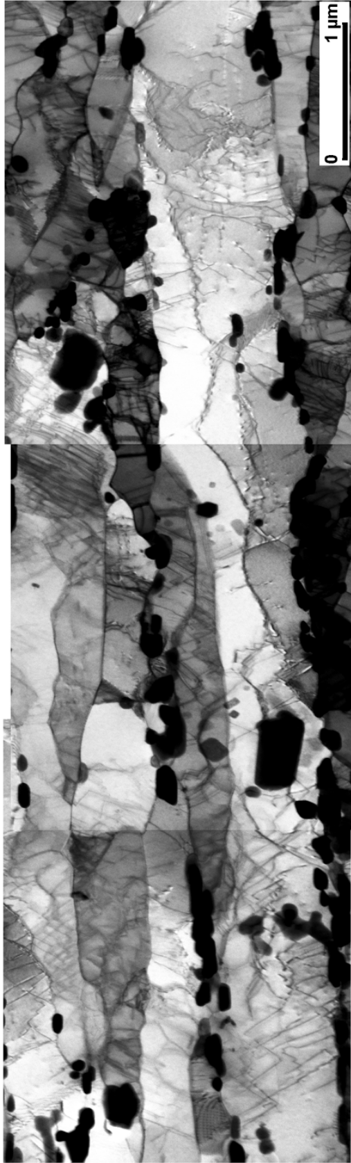
Abbildung 20: 6A microstructure after heat treatment.
