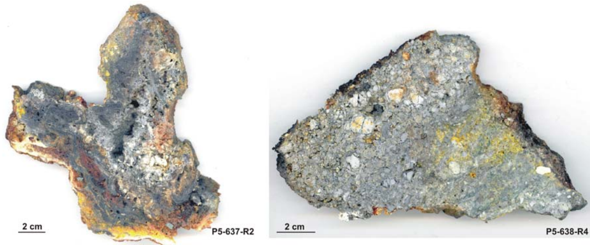
Fig 6.5: Hydrothermal induration and argillic alteration of volcaniclastic sediment -
