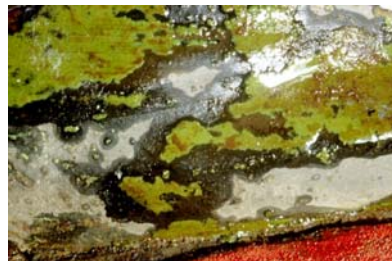
Fig. 6. F-005/00; spots on green (malachite); glossy "coating"
