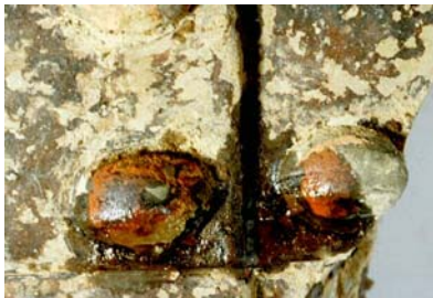
Fig. 4. F-005/00 Spots forming on and around the applied button-shaped stitches of the armour
