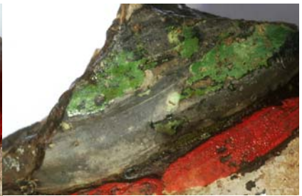
Fig. 29. The green collar in Sept. 2002: the glossy spots form again on the green and the upper fracture edge.
