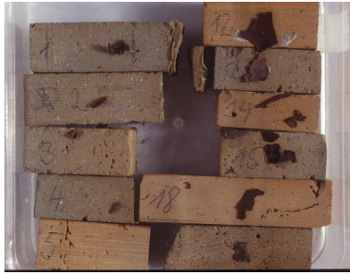
Preliminary test an isolated lacquer flakes on terracotta test slabs
