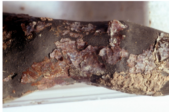
during treatment, detaching lacquer flakes
