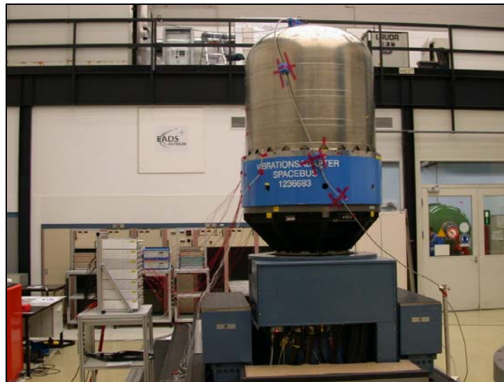
Abbildung 40: Z-Achse on EADS Astrium Test Facility Vertical Test Setup
