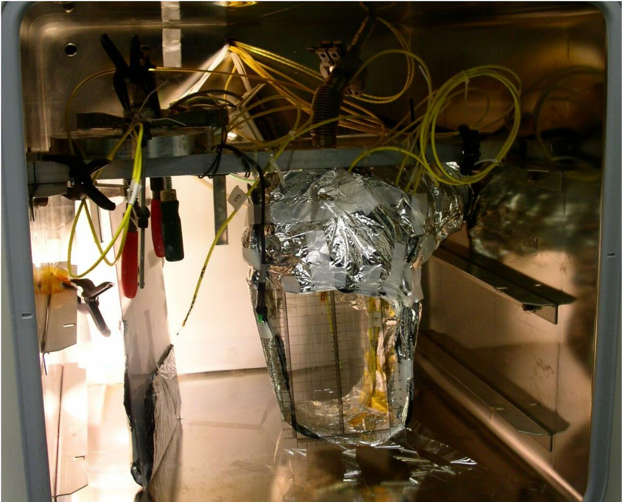
Fig. 33: Glass test vessel inside vacuum chamber. The test chamber is covered with MLI in order to reduce radiative heat, especially from the light source.
