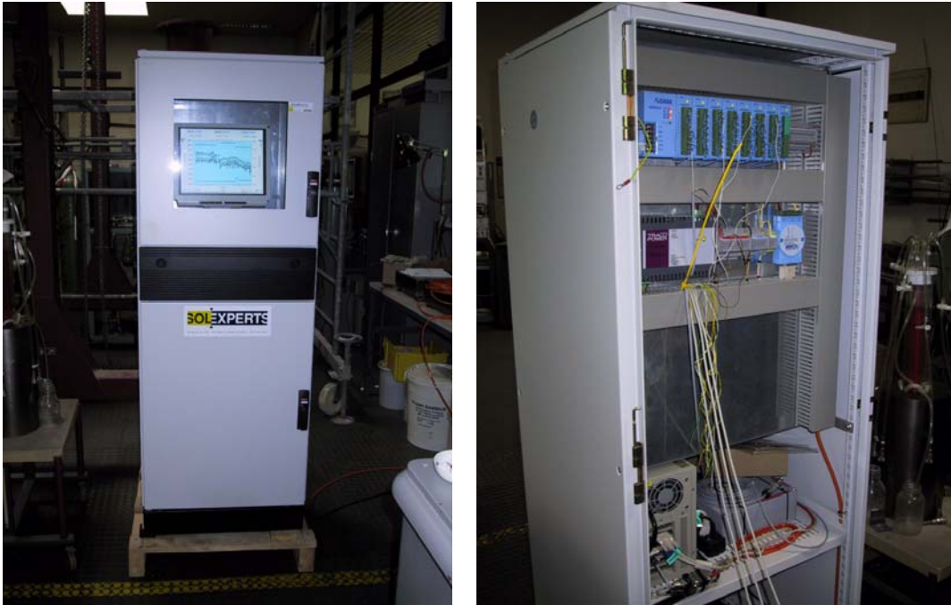
Fig. 3.7 Data acquisition system – front view (left) and rear view (right)
