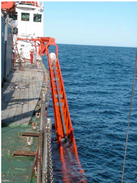
Fig. 5.6.2.: Recovery of a 15 m-Piston Corer during SO201-2
