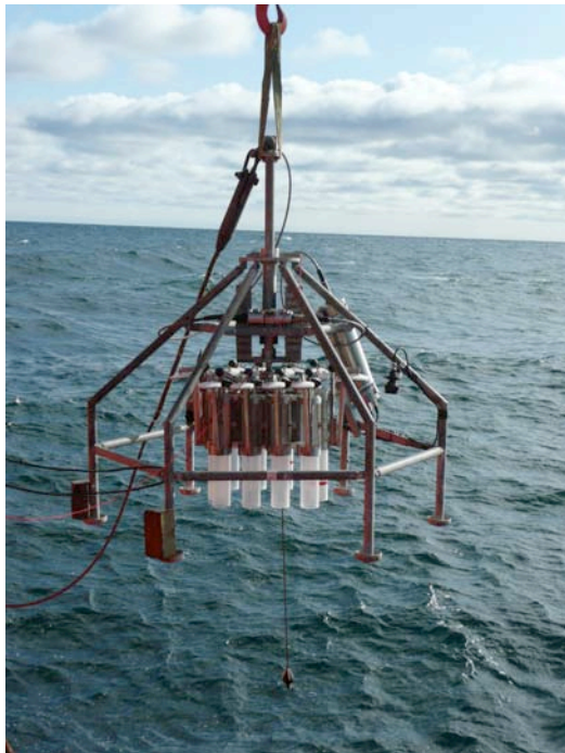
Fig. 5.6.1.: Deployment and retrieval of multicorer mounted with the deep-sea color TV camera system of Fa. Marinetechnik Kawohl.
