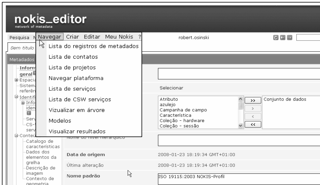
Fig. 2: User interface for creating ISO19115 metadata for the Coastal Zone Metadata Profile
