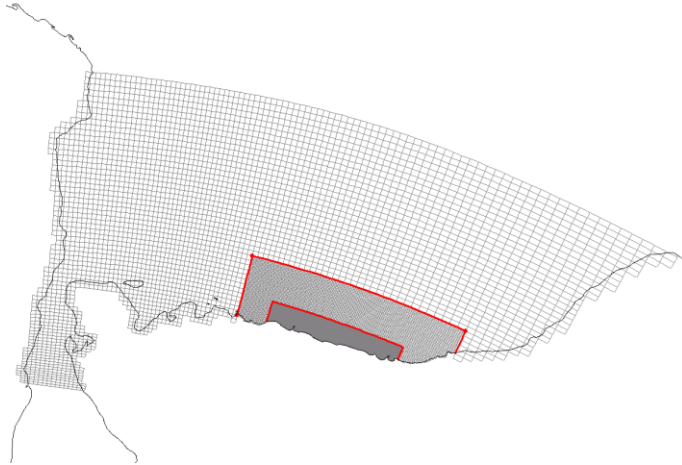
Figure 1.22. Celukanbawang hydrodynamic model grids. Each grid increases in resolution providing a 50 m cell size in the area of interest.
