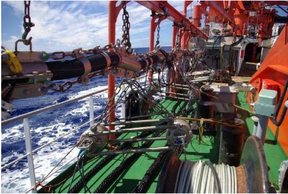
Figure 3.3: G-gun cluster array with 6 airguns in 3 clusters
