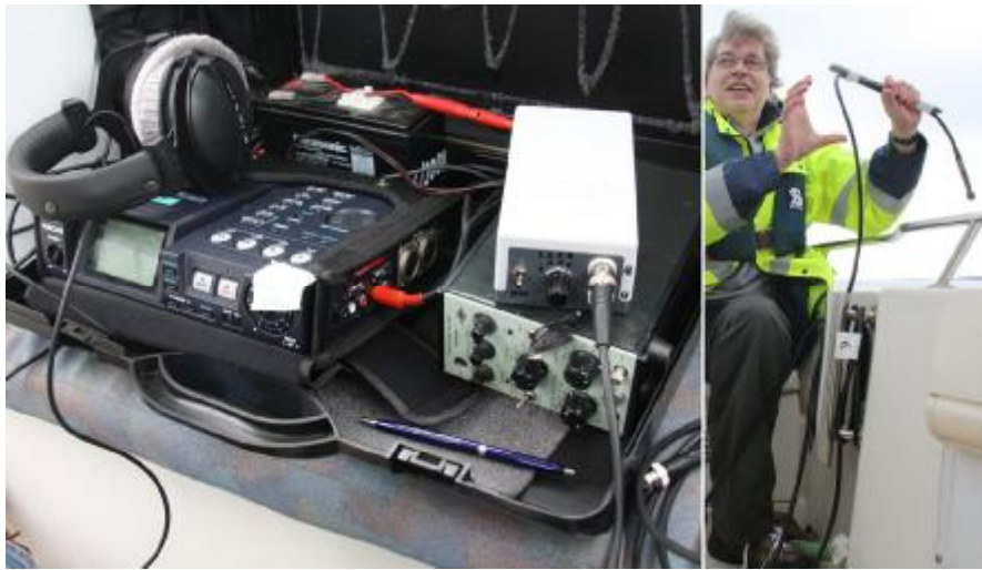
Fig. 6: Recording equipment and hydrophone used at Fyns Hoved
