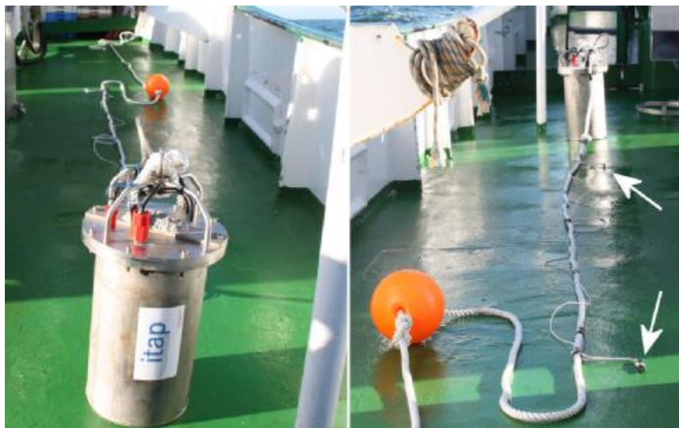
Fig. 4: Measurement system before deployment. The recording electronics is embedded in the cylindrical steel housing. Arrows in the right-hand photo mark the hydrophones.
