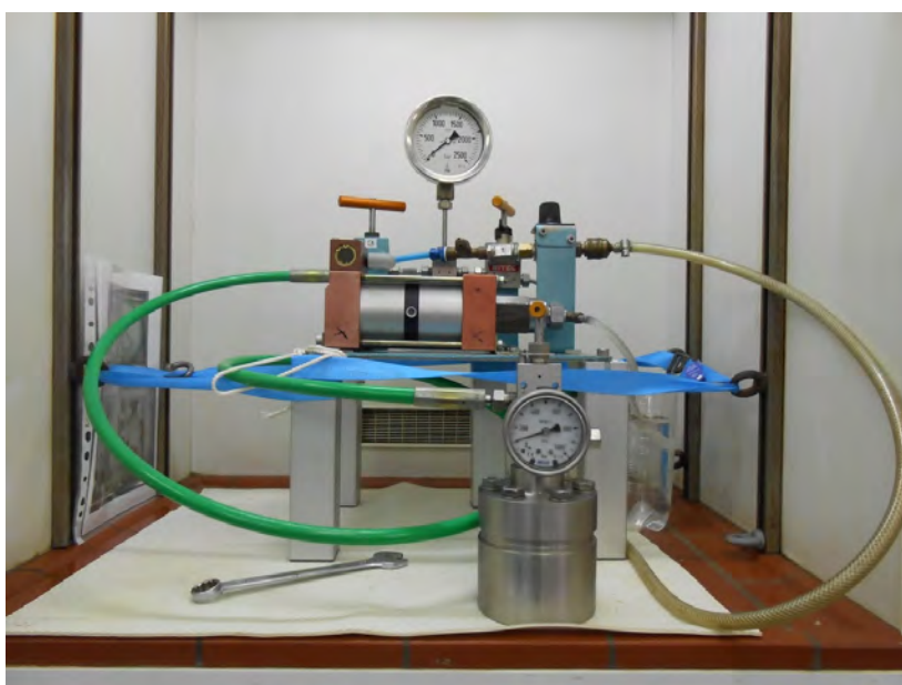
Fig. 9.1 Pressure generating system to expose deep-sea nanofauna at different hydrostatic pressure.
