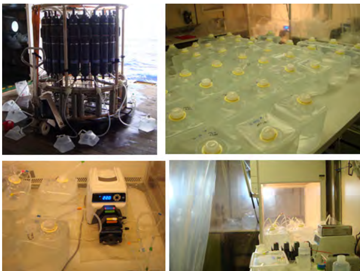
Fig. 4.4 Sampling and filtration of seawater from Niskin bottles (top left) and pre-concentration of REEs (bottom left). Top right and bottom right: 5 L samples and clean-room bubble with pumps.
