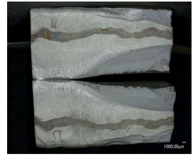
Probe NVEBW 20.1-3 \Delta\sigma = 150 \text{ N/mm}^2 ; N_f = 465.682
