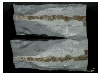
Probe NVEBW 20.2-12 \Delta\sigma = 200 \text{ N/mm}^2 ; N_f = 97.668
