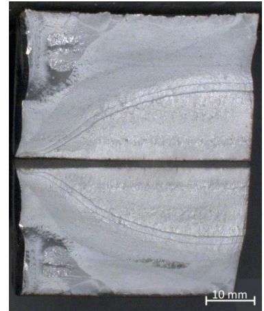
Probe UP 30.3-13 \Delta\sigma = 300 \text{ N/mm}^2 ; N_f = 179.069
