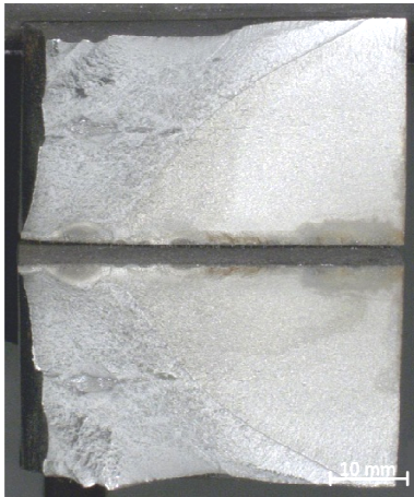
Probe UP 30.3-14 \Delta\sigma = 200 \text{ N/mm}^2 ; N_f = 972.379
