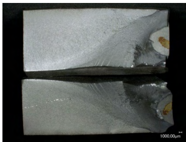
Probe NVEBW 20.1-7 \Delta\sigma = 200 \text{ N/mm}^2 ; N_f = 258.022
