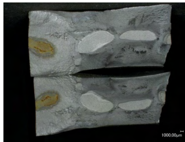
Probe NVEBW 20.1-5 \Delta\sigma = 250 \text{ N/mm}^2 ; N_f = 70.114
