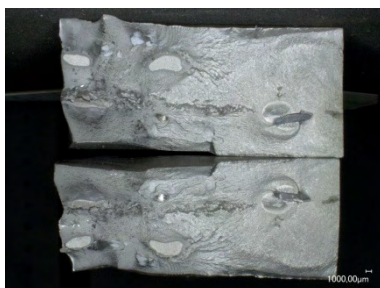
Probe NVEBW 20.2-9 \Delta\sigma = 150 \text{ N/mm}^2 ; N_f = 2.071.805
