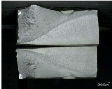
Probe NVEBW 20.1-1 \Delta\sigma = 250 \text{ N/mm}^2 ; N_f = 190.643
