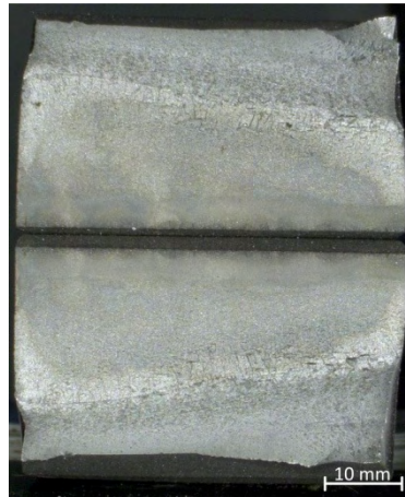
Probe UP 30.3-15 \Delta\sigma = 200 \text{ N/mm}^2 ; N_f = 742.711
