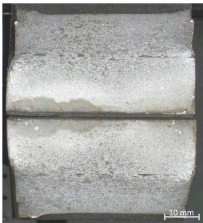
Probe UP 30.3-17 \Delta\sigma = 250 \text{ N/mm}^2 ; N_f = 318.813
