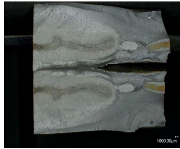
Probe NVEBW 20.1-2 \Delta\sigma = 200 \text{ N/mm}^2 ; N_f = 247.879
