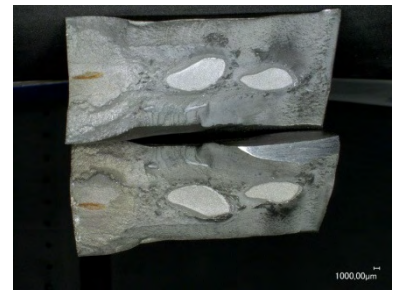
Probe NVEBW 20.1-6 \Delta\sigma = 300 \text{ N/mm}^2 ; N_f = 32.778
