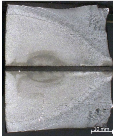
Probe UP 30.3-12 \Delta\sigma = 200 \text{ N/mm}^2 ; N_f = 1.011.817
