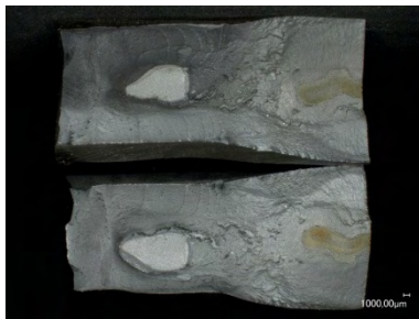
Probe NVEBW 20.1-4 \Delta\sigma = 250 \text{ N/mm}^2 ; N_f = 62.095
