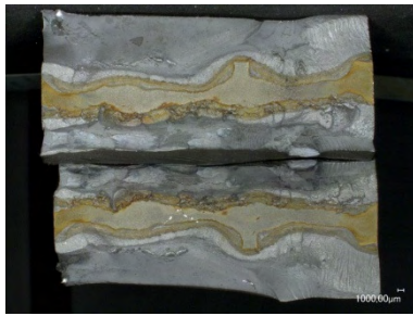
Probe NVEBW 20.2-14 \Delta\sigma = 300 \text{ N/mm}^2 ; N_f = 26.603
