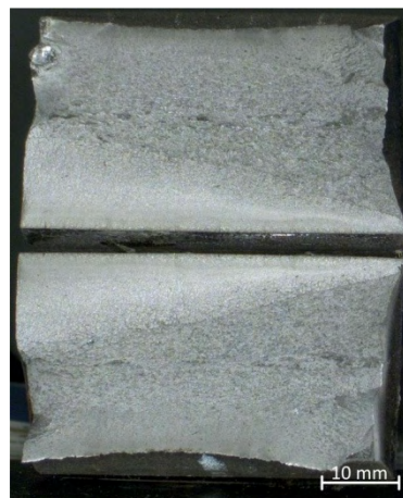
Probe UP 30.3-18 \Delta\sigma = 300 \text{ N/mm}^2 ; N_f = 92.099
