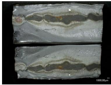
Probe NVEBW 20.2-15 \Delta\sigma = 200 \text{ N/mm}^2 ; N_f = 147.809
