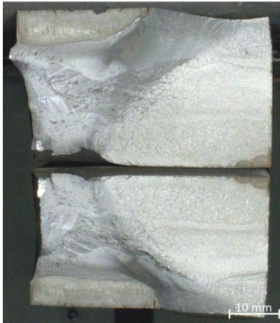
Probe UP 30.3-10 \Delta\sigma = 250 \text{ N/mm}^2 ; N_f = 419.349
