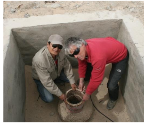
Fig. 5: View on the borehole casing of SG-1B. After the initial drilling campaign to 550 m, the borehole was kept open and intact in order to allow a later deepening as part of this pilot study. Eventually, a final depth of 723 m was reached.
