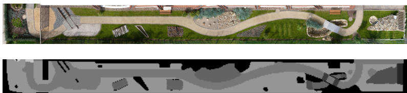
Fig. 4 Up: photo of our outdoor test track at DFKI. Down: the hand-made classification per terrain type. Terrain types are internally associated with average speed values. The cost is time to travel.
