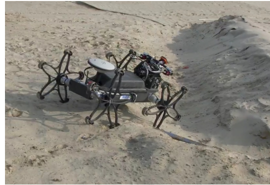
Fig. 1. The Asguard v3 [4] platform has a similar mechanical design compared to the Asguard v2 [13], but includes additional sensors and on-board processing. The main sensors used for this work are the wheel and joint encoders and an IMU. An RTK GPS was used for providing reference measurements.
