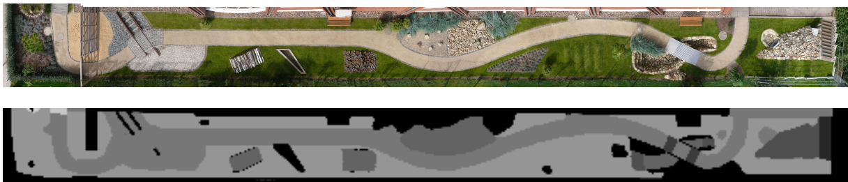
Figure 2: Up: photo of our outdoor test track at DFKI. Down: the hand-made classification per terrain type. Terrain types are internally associated with average speed values. The cost is time to travel.
