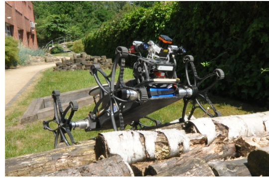
Fig. 4. The Asgard v3 [17] platform has a similar mechanical design compared to the Asgard v2 [18], but includes additional sensors and on-board processing. The main sensors used for this work are the wheel and joint encoders and an IMU, as well as the laser range finder.
