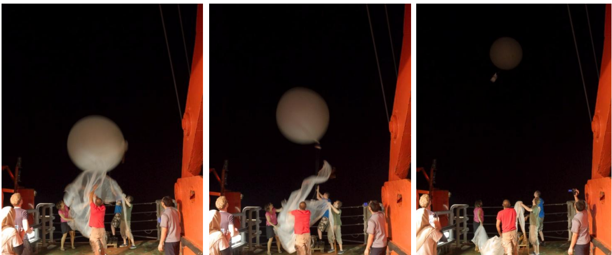
Figure 5: Release of an ozone-sonde at night (photos: Johannes Lampel).
