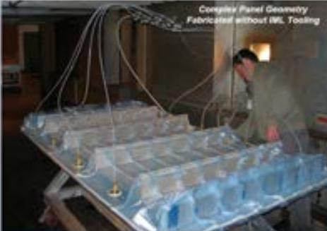
Complex Panel Geometry Fabricated without IMJ Tooling
