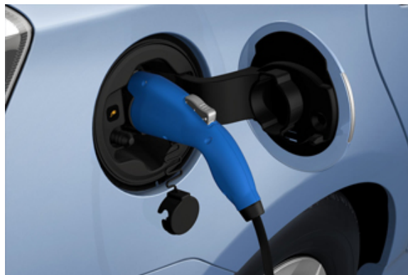
Figure 41 Battery charging system for Toyota PHEV Source Toyota Motor Corporation (2012c)
