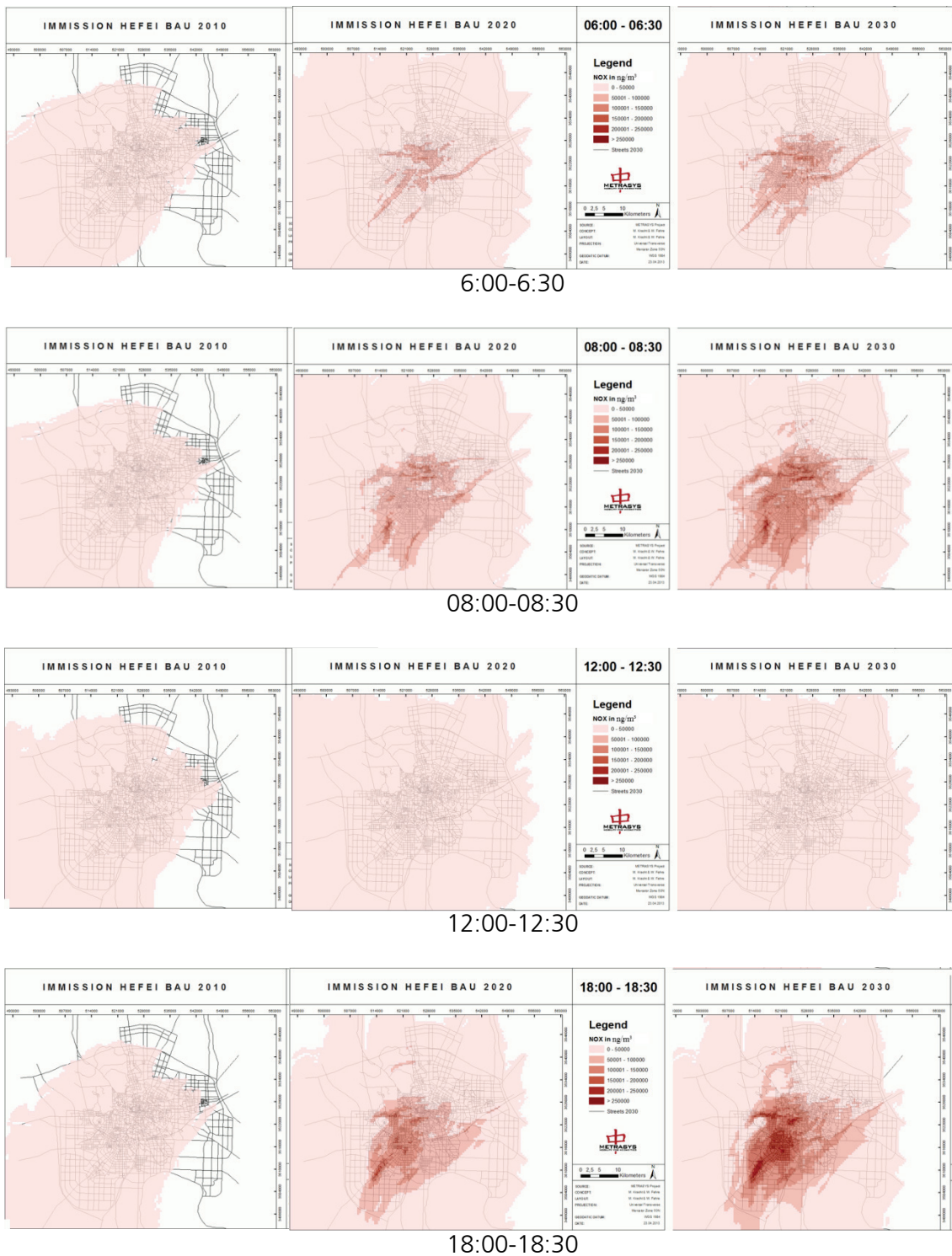
Figure 12: Immissions for the BAU scenario for the year 2010, 2020, 2030 (example NO x ); source: METRASYS
