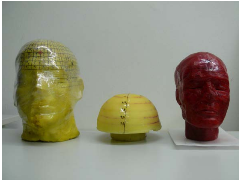
Figure 2.4.2: Head phantoms used for the HMGU PBC calibration: USTUR case 102 phantom, CSR phantom and BFS phantom, from left to right.
