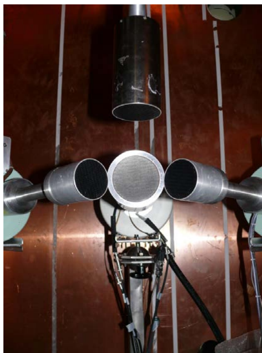
Figure 2.4.1: Partial body counter germanium detectors in skull measurement geometry configuration, on the right detector 2, on the left detector 3, in the middle detector 4, on the top detector 6.
