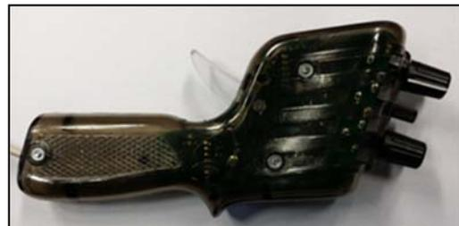
Figure 1: Handset control for continuous recording of comfort
