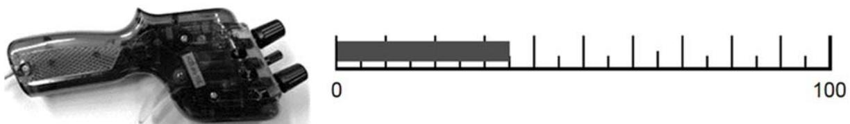
Figure 1: Handset control (left) and visual feedback (right) for the online-measurement of driving discomfort while driving highly automated. Higher values indicate higher discomfort.
