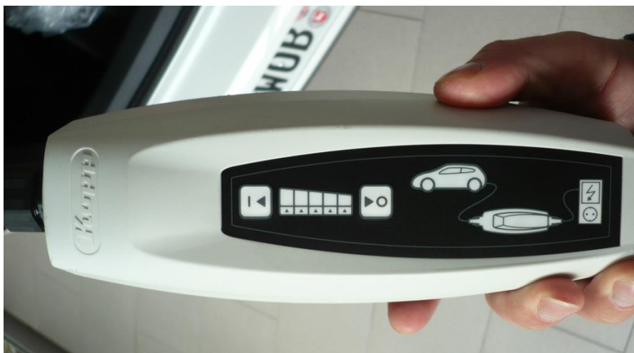
Abbildung 2.2: In Cable Control and Protection Device (IC-CPD)
