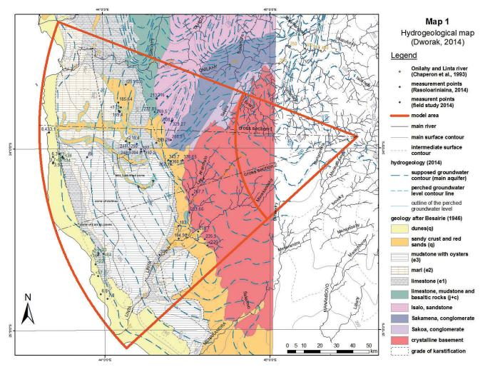
Figure 16: Map of the hydrogeological large-scale model showing the different geological units together with groundwater levels for the model area (Dworak, 2014).
