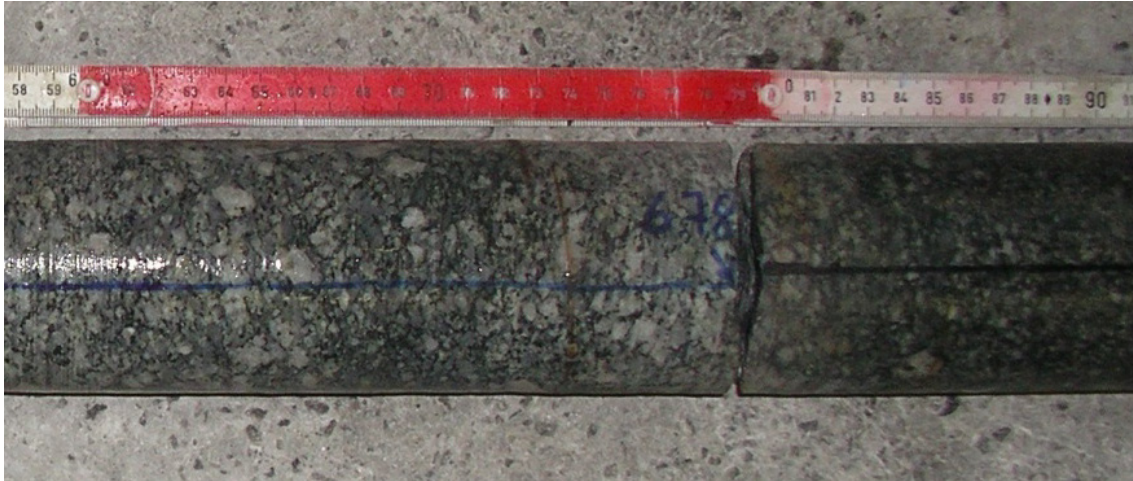
Figure 2.39: Photograph of the core section from borehole CFM 06.002 showing the fracture plane at a depth of 6.78 m. To account for localisation difficulties the key feature is generally considered to be in the depth range of 6.70 – 6.85 m.
