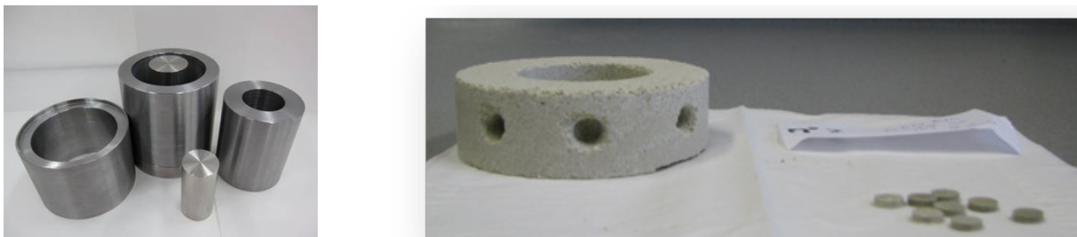
Figure 2.17: (left) Different molds manufactured by CIEMAT for compaction of bentonite rings. (right) Compacted bentonite ring ( 1.65 \text{ g}\cdot\text{cm}^{-3} ) with 8mm drilled holes for emplacement of glass vials. In the lower right region of the image pellets of 2mm thickness are shown to close the pre-manufactured holes.
