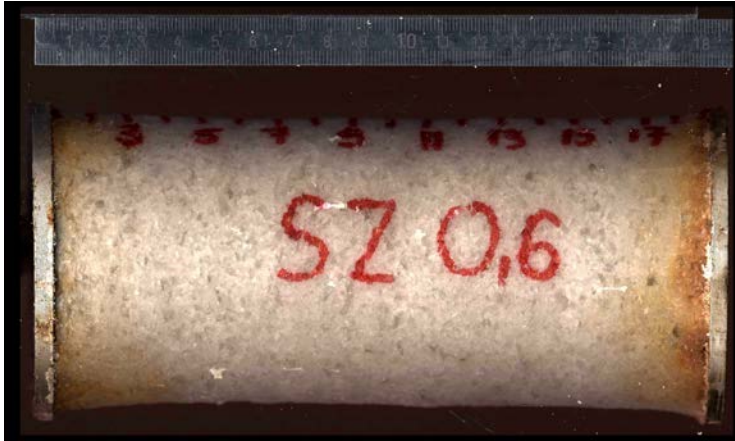
Fig. 2.24 Sample with 0.6 % initial moisture content after dismantling
