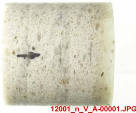
Fig. 2.40 Crushed salt core D-OE-099/1 after the “dry” compaction/permeability test
