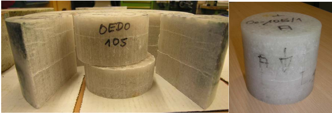
Fig. 2.45 Crushed salt core D-OE-105/01 with sample remains, and the core after the triaxial compaction/permeability test
