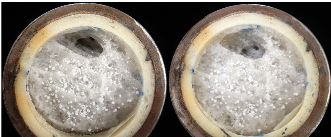
Fig. 2.51 Sample M2a after some dissolution in boiling water.
