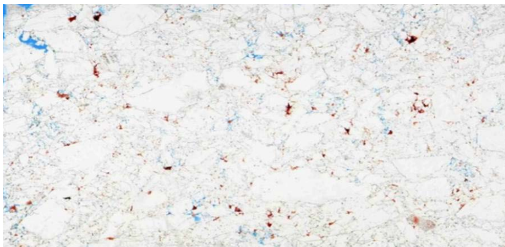
Fig. 2.63 Thin section images (120x55 mm) of the crushed salt sample D-A-25/2 initially compacted in a dry state and subsequently permeated with brine
