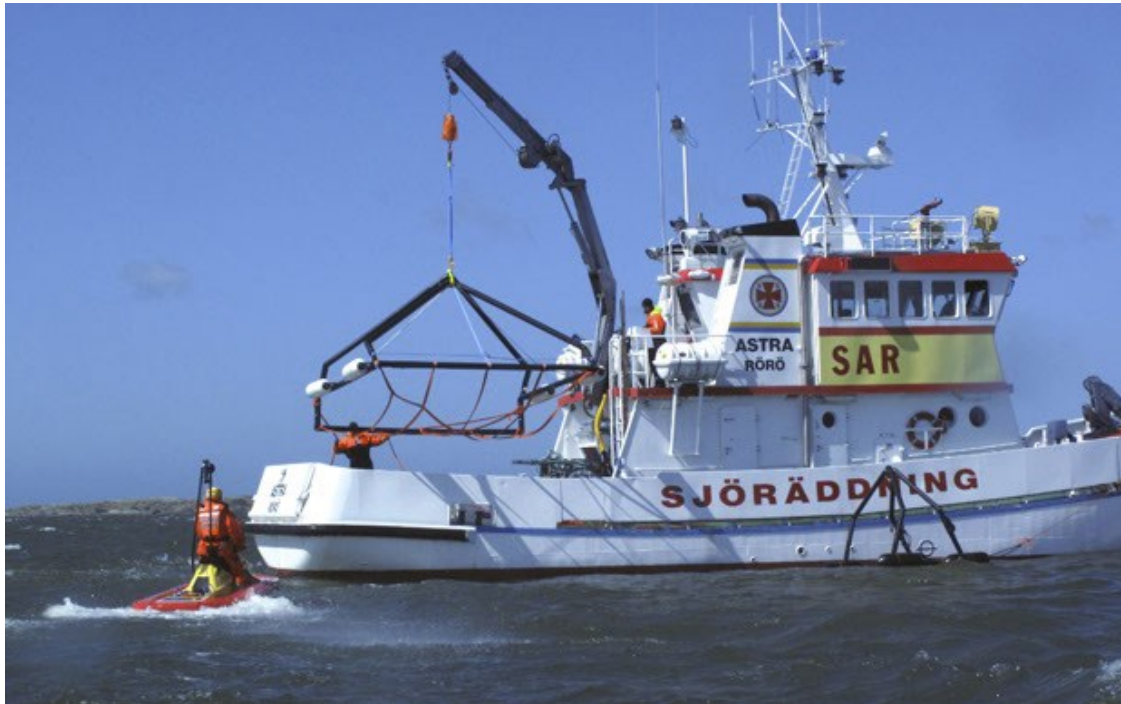
Abbildung 9: Liferaft Recovery cradle System, Foto: www.first-rescue.org
