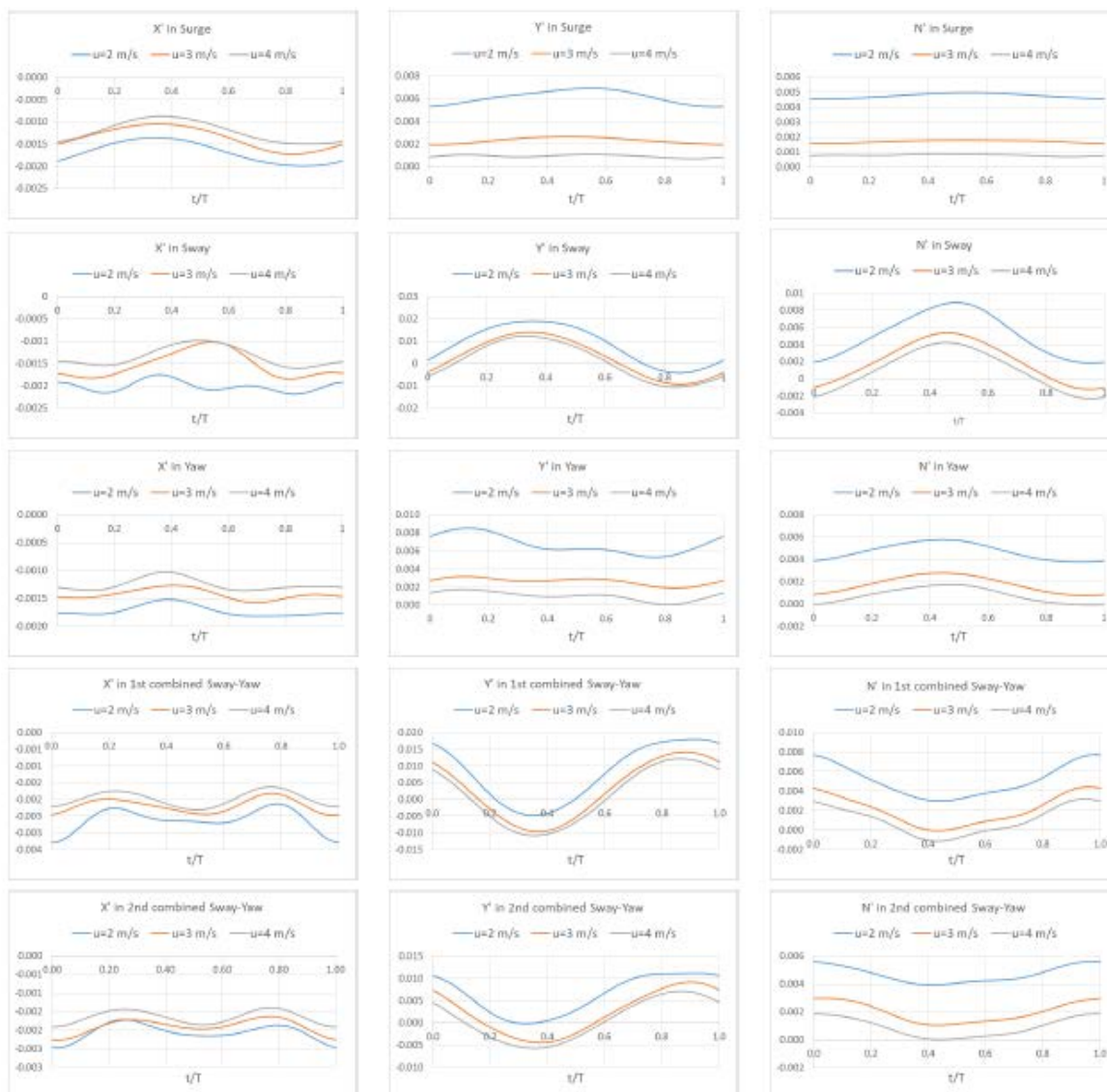
Fig. 5.43: Comparison of non-dimensional forces and moment of three velocities in the forced dynamic motion with working tunnel thruster (from top to bottom: surge, sway, yaw, 1st and 2nd combined sway-yaw test)
