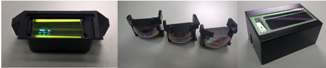
Figure 4.5: Transiving optics (left), coated receiving lenses (middle) and coated housing (right) for 1550 nm
