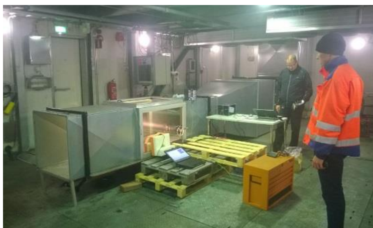
Figure 4.1: Fog chamber for LIDAR testing.
