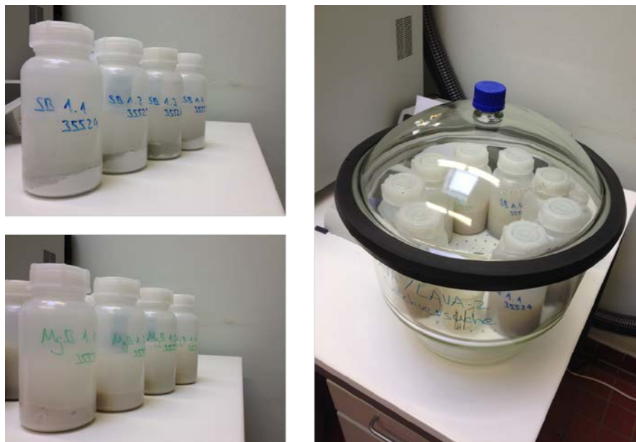
Fig. 4.1 Preparation of batch experiments in PE-bottles (left) and storage of PE-vessels in exsiccator (right)
