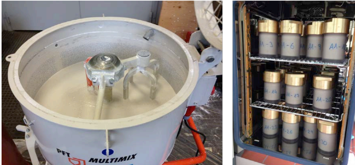
Fig. 3.2 Production of sorel concrete A1 in laboratory: Mixing of sorel concrete in compulsory mixer (left) and hardening of samples in air tide vessels in climate cabinet (right)
