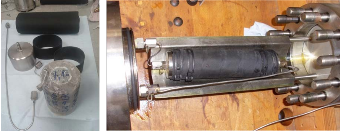
Fig. 4.44 Installation of the combined sample in the isostatic cell with rubber jacket
