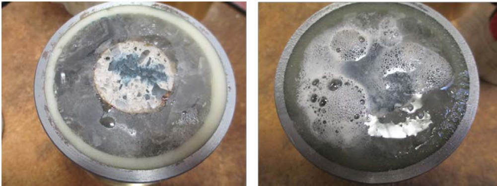
Fig. 4.60 Verification of the contact seam between salt concrete and rock salt after dismantling from isostatic cells. Left: Saline solution pathed the samples driven by compressed air (Core 4). Right: Visualization of path ways using leakage spray (Core 5)
