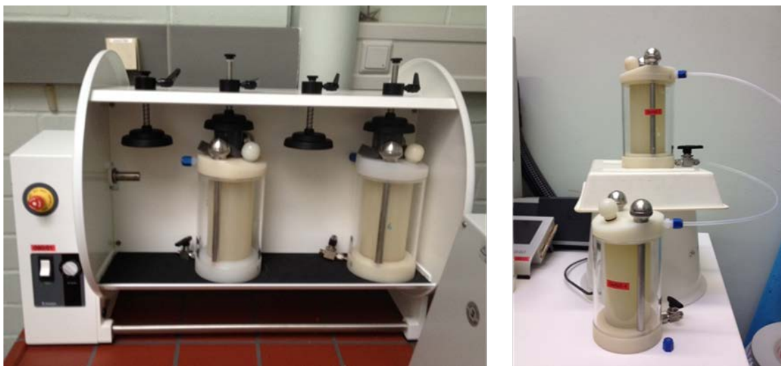
Fig. 4.23 Execution of cascade experiment in laboratory: pressure vessels in overhead shaker (left) and separation of reacted solution from concrete at the end of cascade (right)
