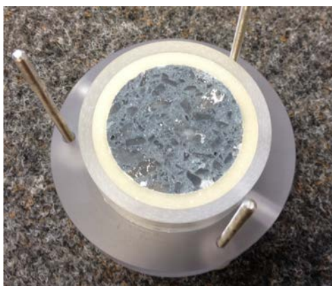
Fig. 4.32 Concrete sample inserted in the lower part of a diffusion cell. Concrete sample was inserted in an acrylic glass tube and afterwards cast in araldite
