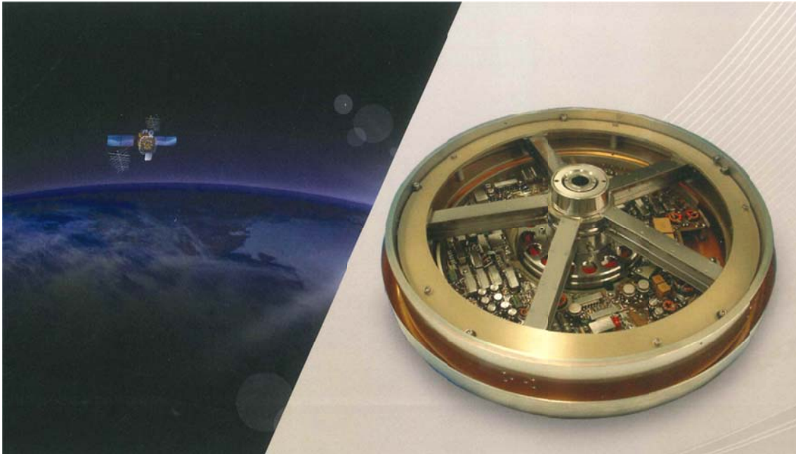
Abbildung 12: Rockwell Collins Wheel 2: HAT-RSI High Motor Torque Momentum and Reaction Wheels 12-68 Nms mit integrierter Steuerelektronik ( https://www.rockwellcollins.com/Products-and-Services/Defense/Platforms/Space/High-Motor-Torque-Momentum-and-Reaction-Wheels.aspx ).
