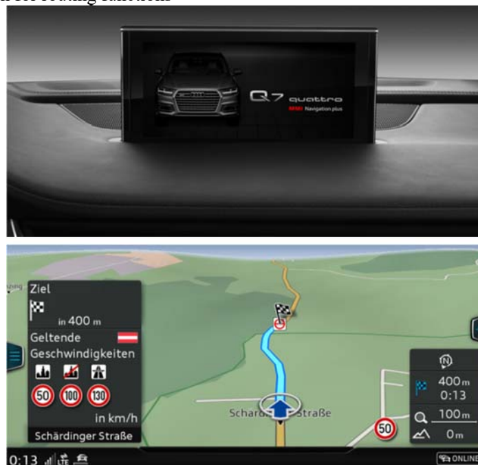
Figure 4.1-7: MMI display - the top shows the installation location, the bottom a typical navigation screen
