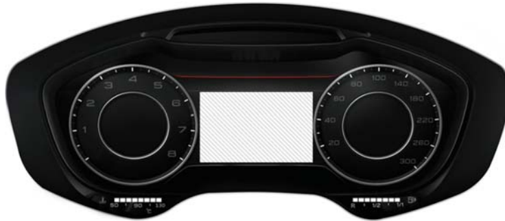
Figure 4.1-8: Audi instrument cluster – the hatched area describes the available space for displaying information in the project.
