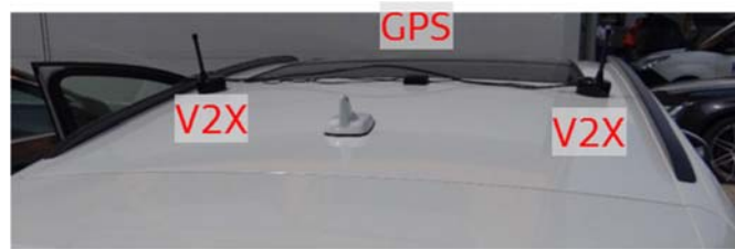
Figure 4.1-10: reference antenna system
