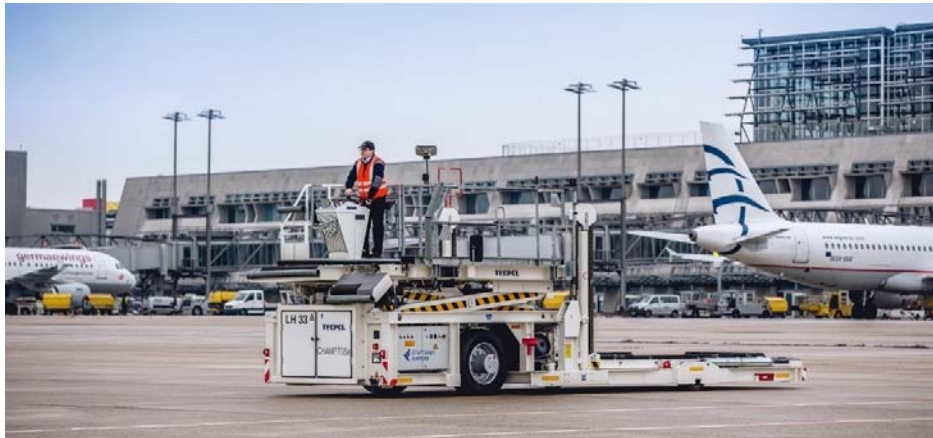
Abbildung 3-9: El. 7t. Highloader, Typ: Champ 7, Trepel Airport Equipment GmbH
