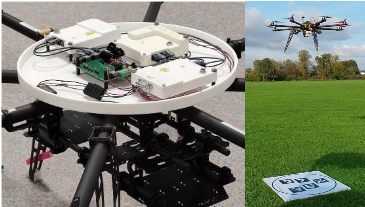
Figure 36: The Volocopter scaled demonstrator used in flight testing
