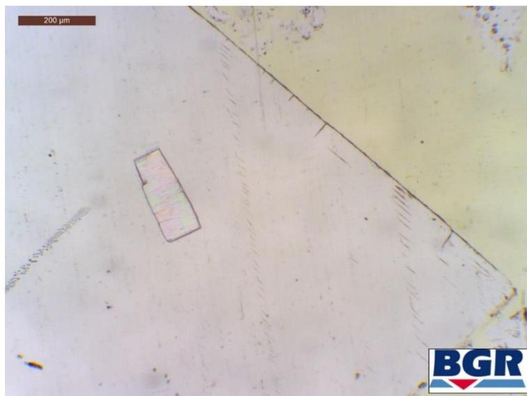
**Fig. 4.4** Halite grain in uncompact crushed salt with en-échelon, a fluid inclusion plane and a grain of anhydrite as a fluid inclusion, scale bar is 200 μm
