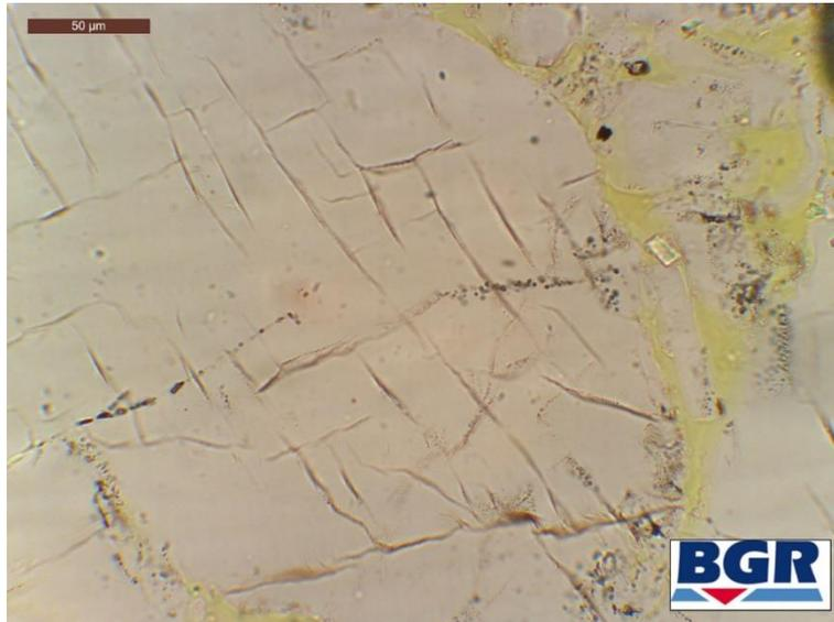
**Fig. 4.50** Halite grain compacted crushed salt with intragranular fractures (microcracks), scale bar is 50 μm
