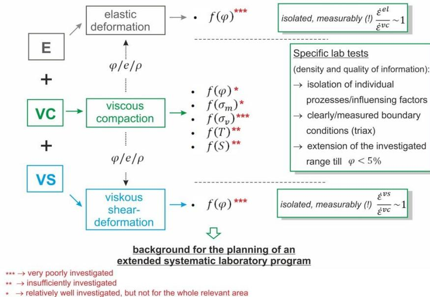
**Fig. 6.24** Schematic representation of the main factors characterizing the THM behaviour of crushed salt and the need of the validation of accordingly functional relationships in the constitutive model approaches
