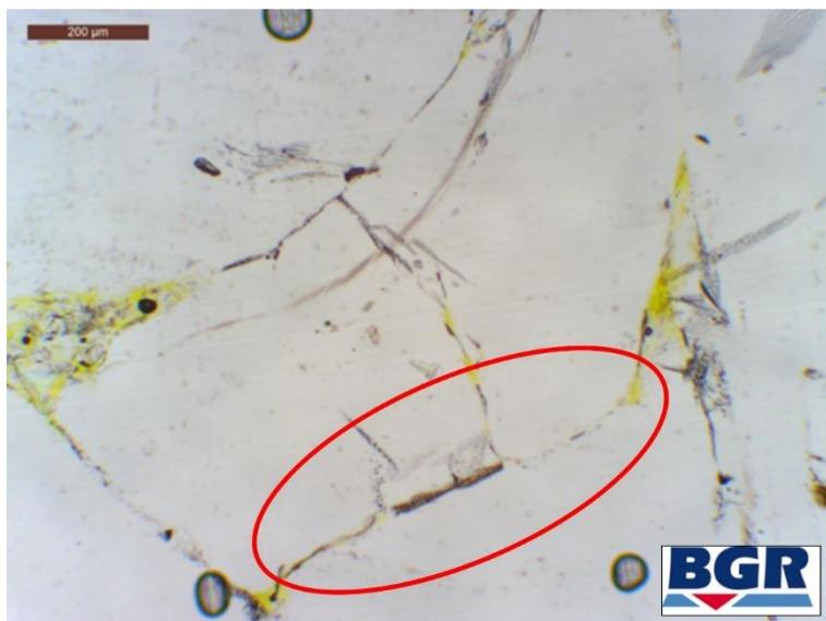
**Fig. 4.56** Indicators for grain boundary diffusion (rounded grain edges with even grain contact, red circle) and compaction fringes in compacted crushed salt, scale bar is 200 μm
