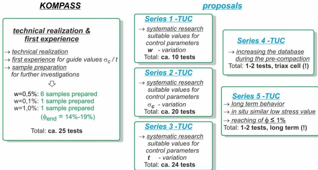
**Fig. 6.3** Overview of the performed and planned investigations on the pre-compaction of crushed salt under in-situ similar stress conditions in fast motion
