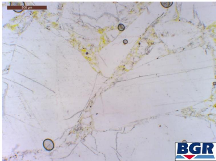
**Fig. 4.58** Bended grain boundaries which are indication for intracrystalline plasticity, in compacted crushed salt, scale bar is 500 μm
