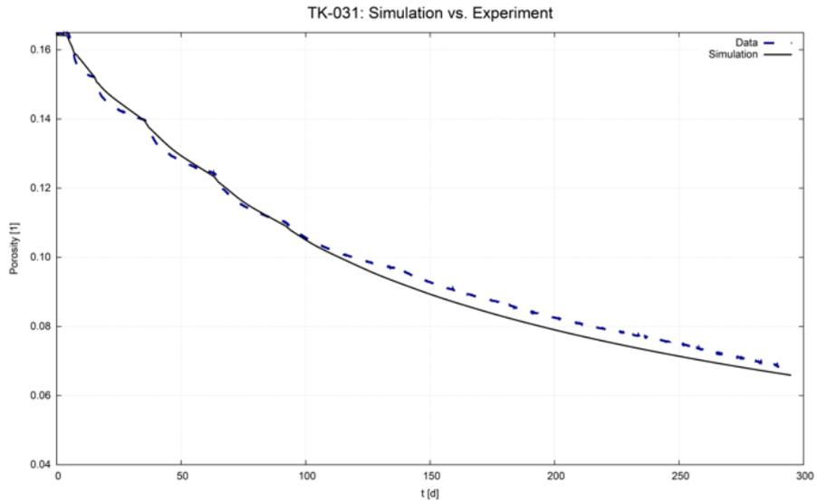
**Fig. 5.37** Simulated porosity evolution vs data for TK-031
