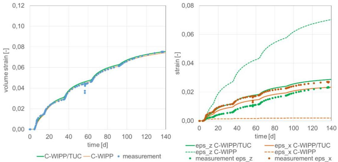
**Fig. 5.55** Recalculation of the volumetric strain and the individual strain components in the TK-031 experiment with the constitutive model C-WIPP/Itasca and with the constitutive model C-WIPP/TUC in comparison
