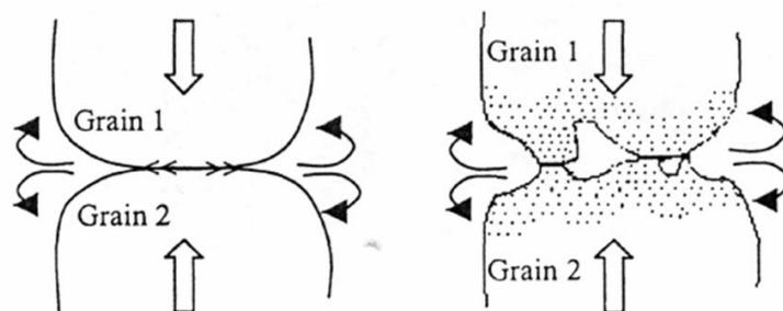
**Fig. 3.8** Schematic representation of pressure solution. Left: Grain boundary diffusional pressure mechanism; Right: Plasticity-coupled pressure mechanism with plastically-deformed region shaded. Figure taken from /HAN 14/
