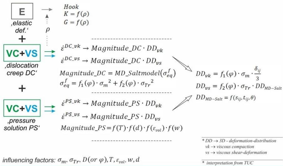
**Fig. 5.19** Structural sketch for the constitutive model Callahan used from Sandia SNL
