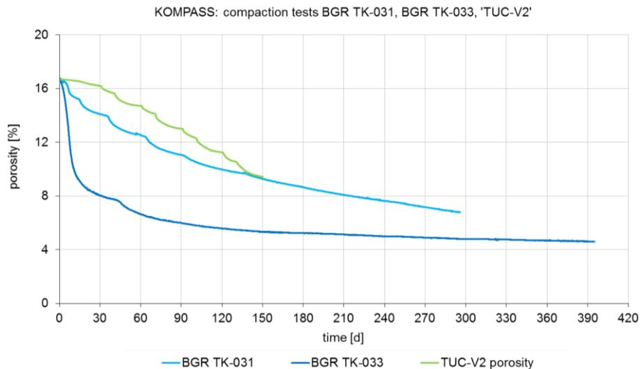
**Fig. 5.57** Measurement results of tests TK-031, TK-033 of BGR and TUC-V2 in comparison (in terms of porosity change)
