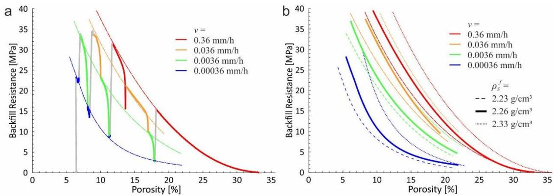
**Fig. 4.12** Load resistance versus porosity for the oedometer test Oedo-112
