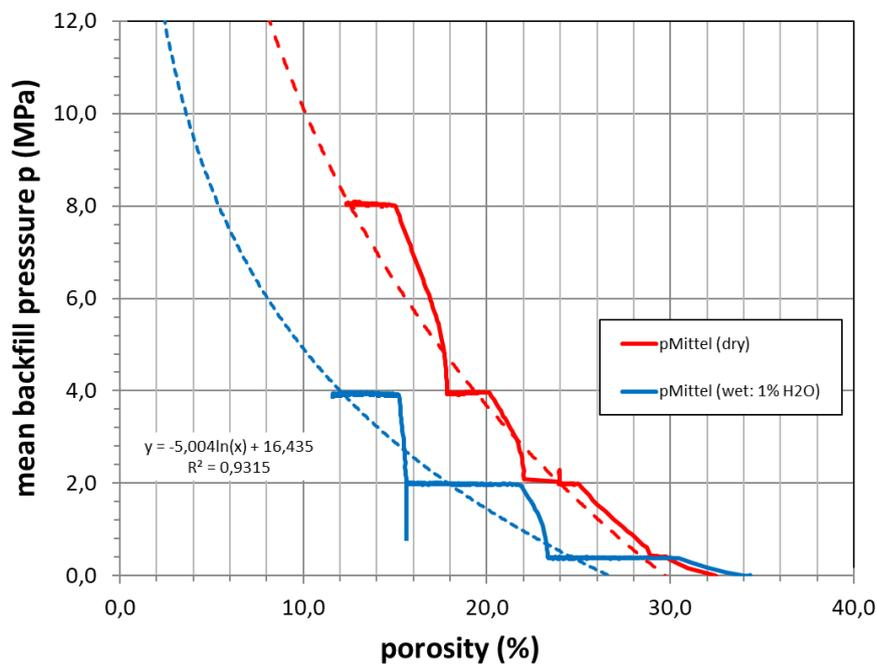
**Fig. 4.34** Backfill pressure vs. porosity (pre-tests with dry and wet conditions)
