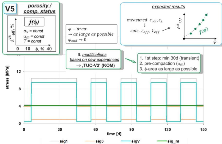
**Fig. 6.13** Loading history of test type V5b, modified
