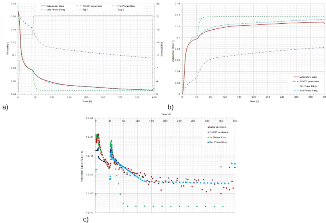
**Fig. 5.34** Evolution of a) porosity, b) volumetric strain and c) strain rate for the simulation of TK-033 with the parameter set developed for TK-031 (dark blue), for the modelling of the first load phase (green) and the second load phase (light blue)
