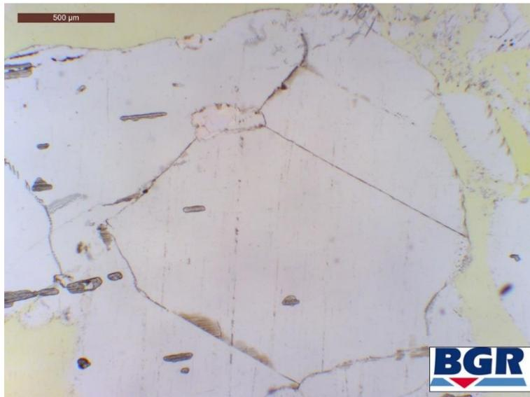
**Fig. 4.8** Halite grain in uncompacted crushed salt with a grain of anhydrite as inclusion, surrounded by intragranular fractures, scale bar is 500 μm
