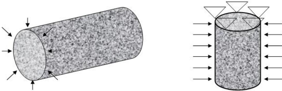
**Fig. 4.14** Schematic sketch for the transfer of the in-situ stress of crushed salt in a section (left) to the triaxial stress of a cylindrical test specimen in an autoclave (right)
