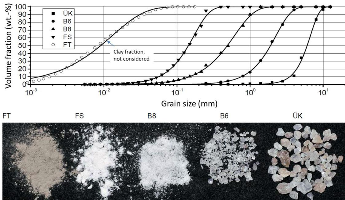
**Fig. 4.3** Salt grain fractions and grain size distributions
