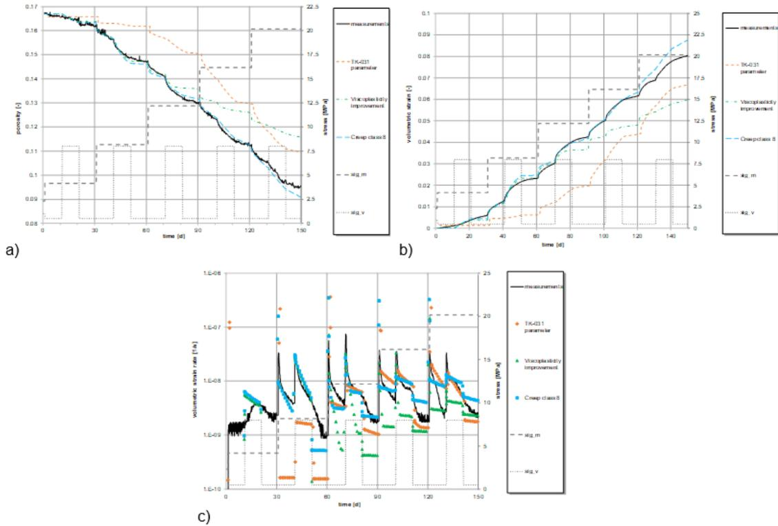
**Fig. 5.35** Evolutions of a) porosity, b) volumetric strain and c) volumetric strain rate for TUC-V2 with the parameter set of TK-031, a viscoplasticity improved and a creep class improved parameter set and
