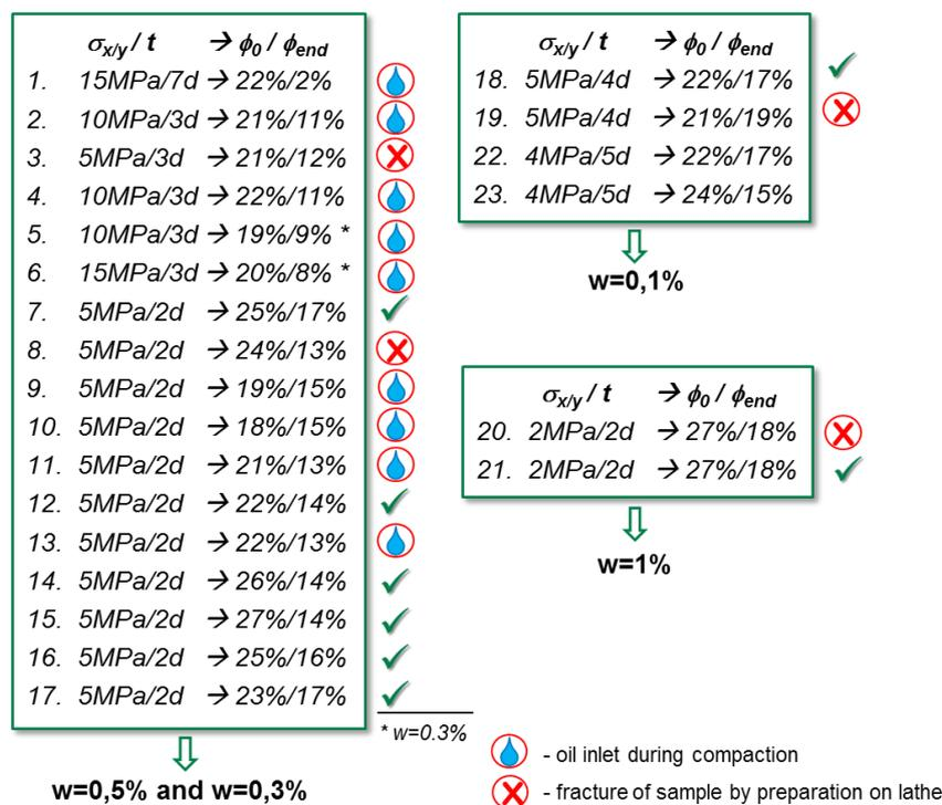
**Fig. 4.24** Compaction tests on classified crushed salt
