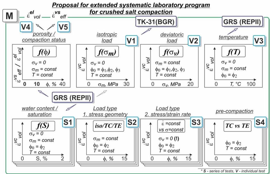
**Fig. 6.7** Second iteration step for planning the laboratory test program
