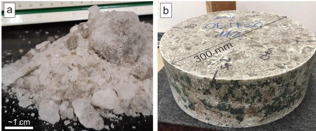
**Fig. 4.9** a) Loose crushed salt from the z2HS formation of the Teutschenthal underground salt mine, b) Test specimen after oedometric compaction
