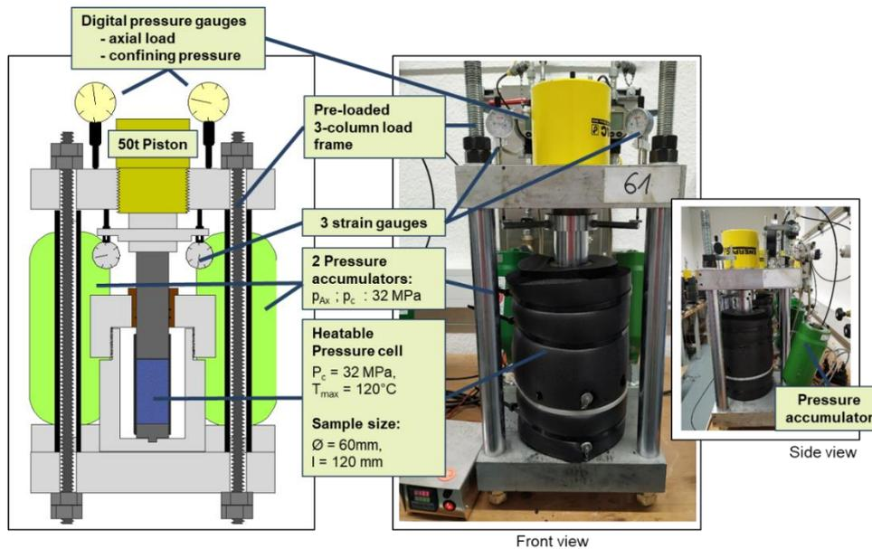
**Fig. 4.41** The long-term creep test device, left: schematic sketch of a hydraulic test rig, right: test rig with heatable triaxial cell
