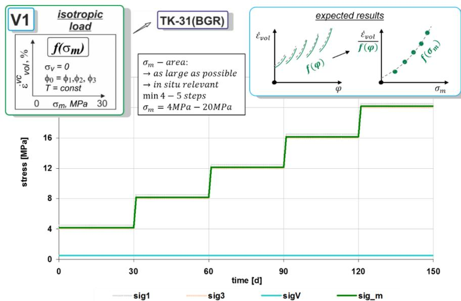
**Fig. 6.8** Loading history of test type V1
