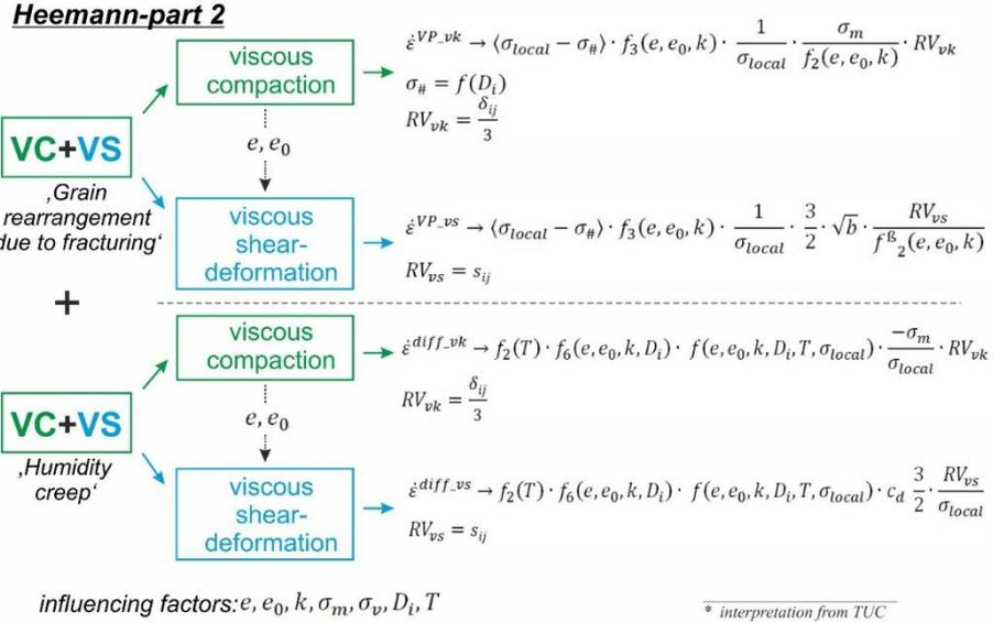
**Fig. 5.22** Structural sketch for the constitutive model Heemann used from BGR
