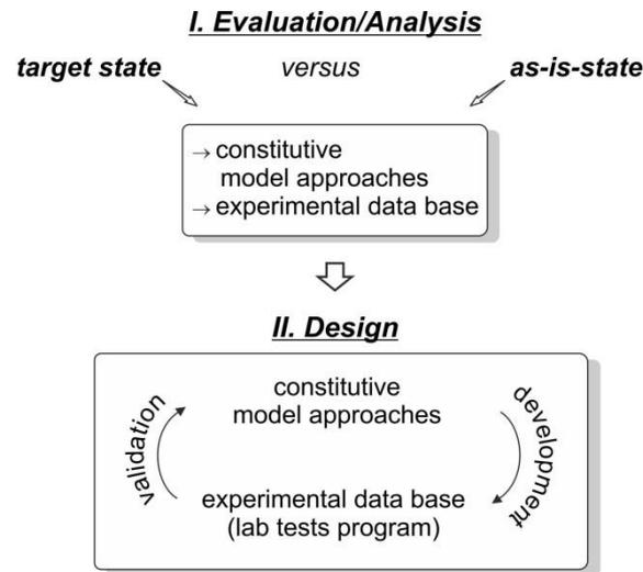
**Fig. 6.25** Main working steps in frame of this project: definition of ‘as-is-state’ and ‘target-state’ in the constitutive modelling for crushed salt, derivation of need for further developments and design of laboratory program to serve this need
