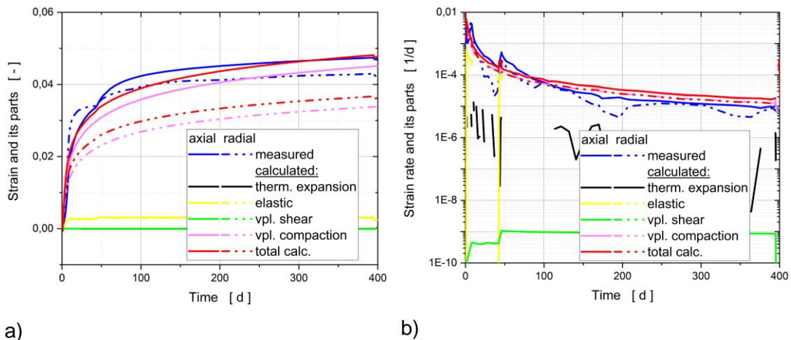
**Fig. 5.24** Measured and calculated deformation behaviour for TK-033, calculation with parameter set TK-033: a) Components of strain in axial and radial direction, b) Components of strain rate in axial and radial direction
