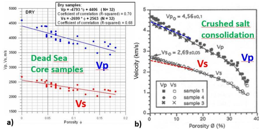
**Fig. 3.3** Ultrasonic wave velocities vs porosity of consolidated halite
