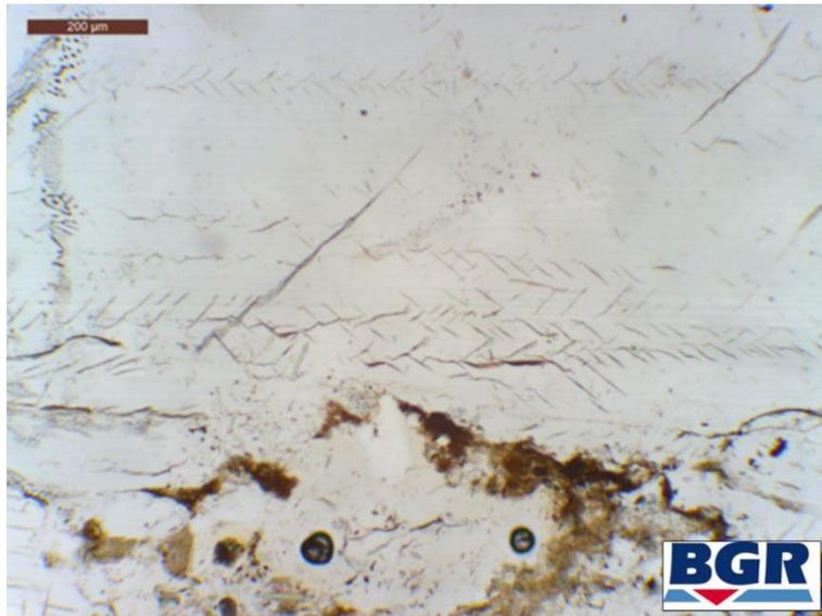
**Fig. 4.51** En-échelon fractures in compacted crushed salt, scale bar is 200  $\mu\text{m}$
