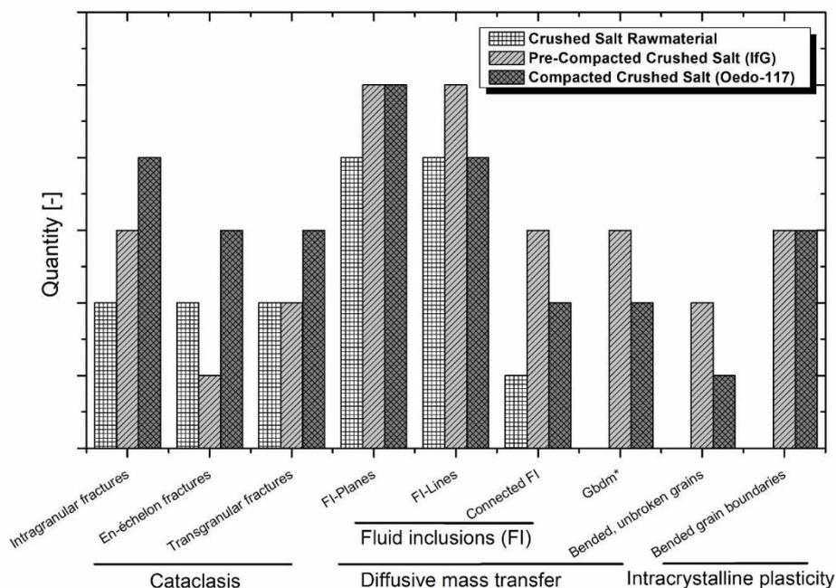
**Fig. 6.1** Observed microstructures in loose crushed salt (two sections) compared to pre-compacted crushed salt (eight sections) and compacted crushed salt (six sections), quantity is just a exclusively value relative to each other.
