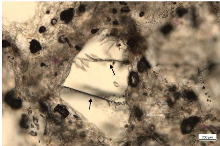
**Fig. 4.47** Sample 681/Oed2 a) Low magnification photomicrograph to observe pore structure and grain shapes and sizes, b) Plastic grain deformation at centre, c) - d) Fluid inclusions in propagated micro-cracks (arrows) in transmitted light
