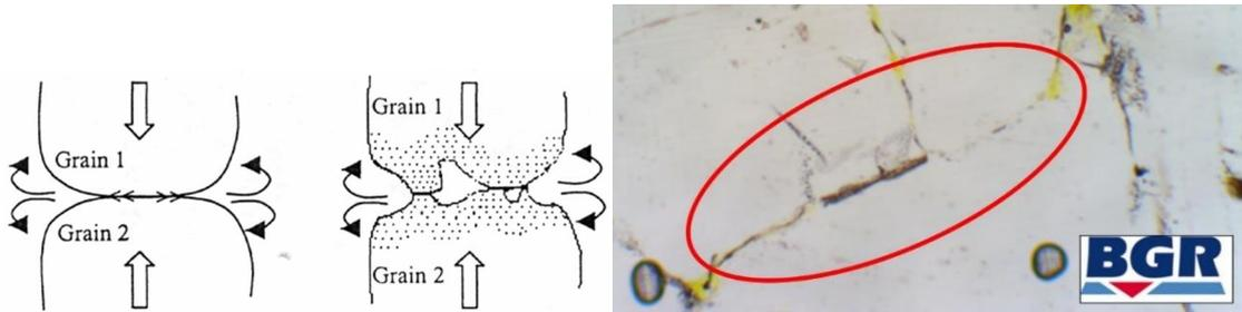
**Fig. 6.2** Visualization of grain boundary diffusion, left: Schematic representation of pressure solution /HAN 14/, right: Microstructural indicators for grain boundary diffusion in a compacted crushed salt sample
