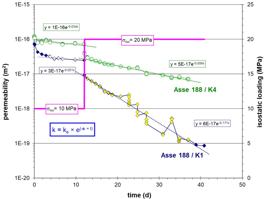
**Fig. 2.2** Gas-permeability decrease of disturbed rock salt as function of time and effective stress /POP 07/
