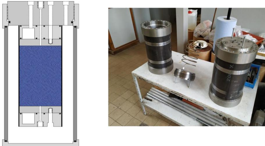
**Fig. 4.60** The new pressure cell developed by IfG
