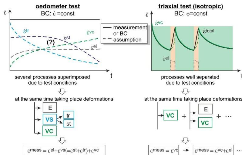
**Fig. 4.2** Comparison sketch of the mechanical processes in an oedometer test and in a triaxial test
