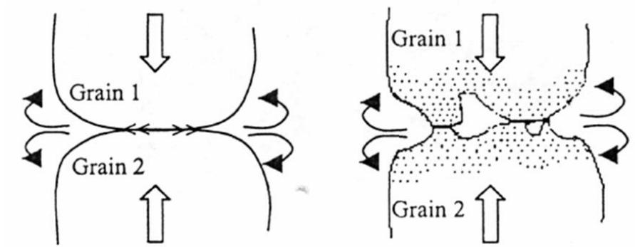
**Fig. 4.57** Schematic representation of pressure solution, left: Grain boundary diffusional pressure mechanism, right: Plasticity-coupled pressure mechanism with plastically deformed region shaded, Figure taken from /HAN 14/
