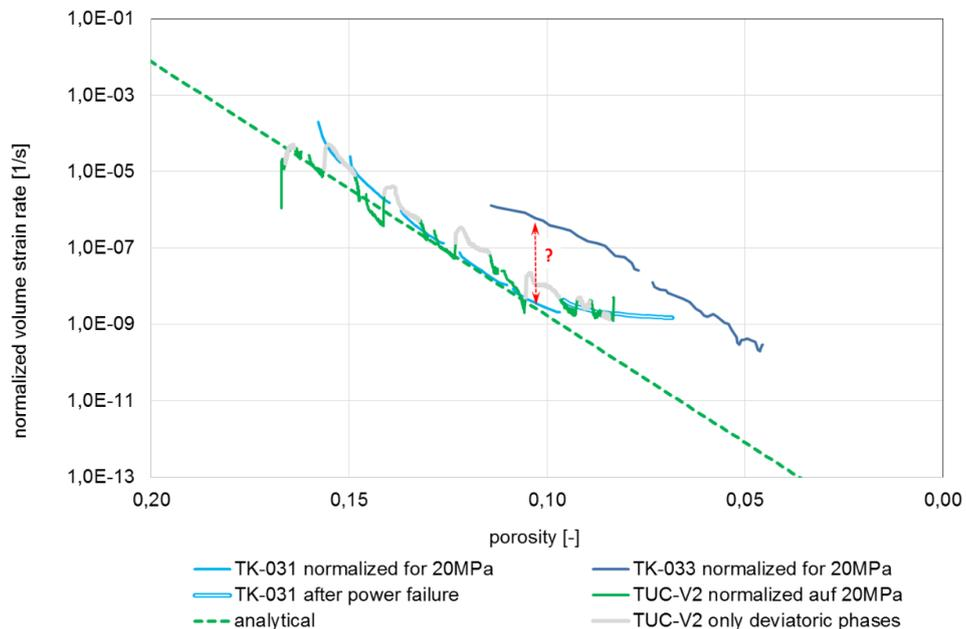
**Fig. 5.58** Normalized measurement results of tests TK-031, TK-033 of BGR and TUC-V2 in comparison (as volumetric strain rates)
