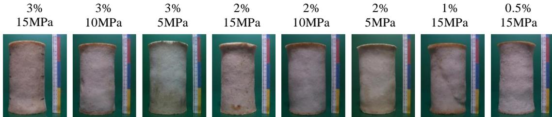
**Fig. 4.19** Preliminary tests on the producibility of pre-compacted crushed salt test specimens
