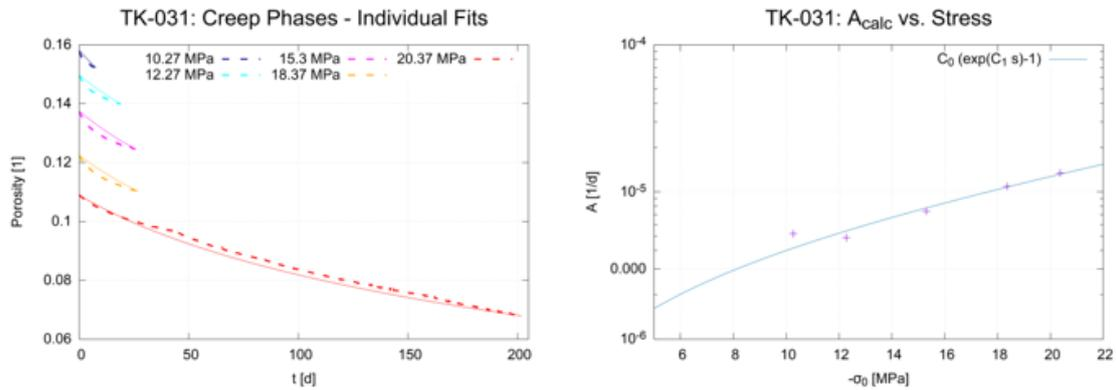
**Fig. 5.36** Intermediate results for TK-031; left panel: Analytic solution for each individual creep phase with  $C_2 = 32.35$  (dashed lines: data, solid lines: simulation); right panel:  $A_{calc}$  (crosses) and  $C_0(e^{C_1 s} - 1)$  (solid line) versus stress for  $C_0 = 3.385 \cdot 10^{-6} / d$  and  $C_1 = 0.078 / MPa$
