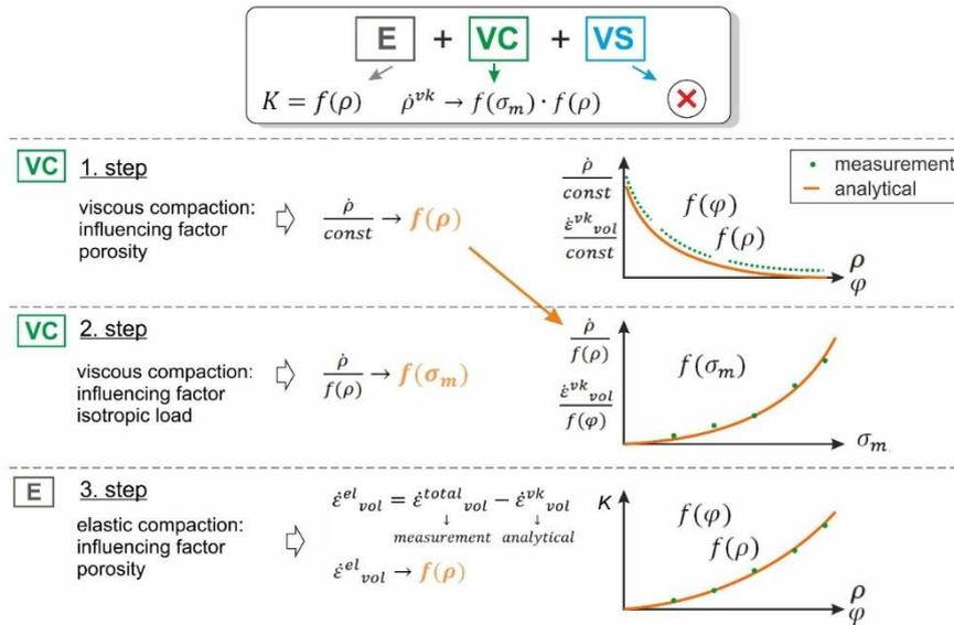
**Fig. 5.52** Schematic sketch of the methodology of the parameter determination for the computational part of the constitutive model C-WIPP/TUC using a multi-stage triaxial long-term test with isotropic load
