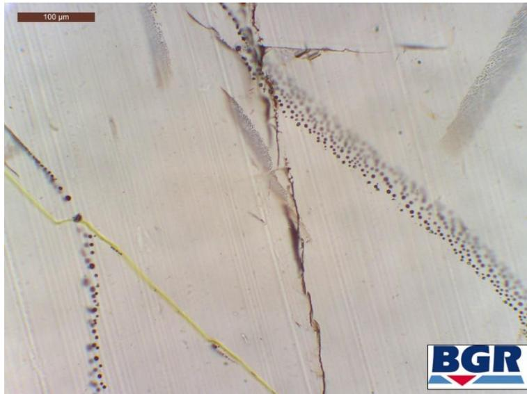
**Fig. 4.7** Halite grain in uncompacted crushed salt with different types of microstructures present, fluid inclusions (planes and lines), en-échelon (centre of the grain) intra- (top of the grain) and transgranular fractures (yellow coloured crack) were observed, scale bar is 100 μm
