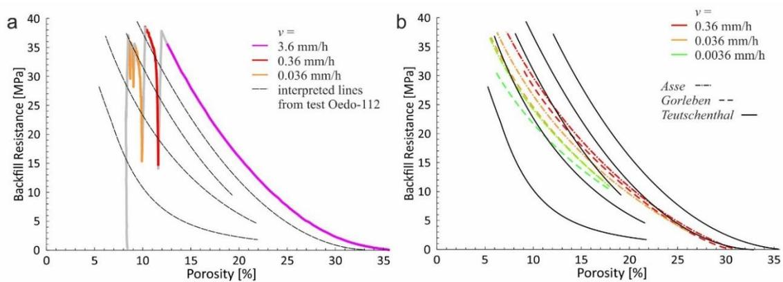
**Fig. 4.13** (a) Load resistance versus porosity values given for differing strain rates (in colour) of test Oedo-113, b) Interpreted lines of crushed Asse and crushed Gorleben salt behaviour at different compaction speeds (in colour) and interpreted lines of Oedo-112 and Oedo-113 (solid black lines)
