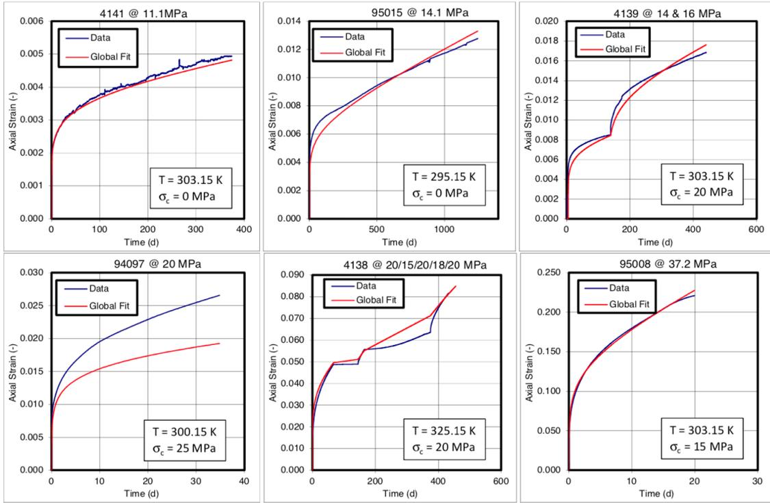
**Fig. 5.40** Comparison of MD model fit and data for intact Asse salt /DEV 11/
