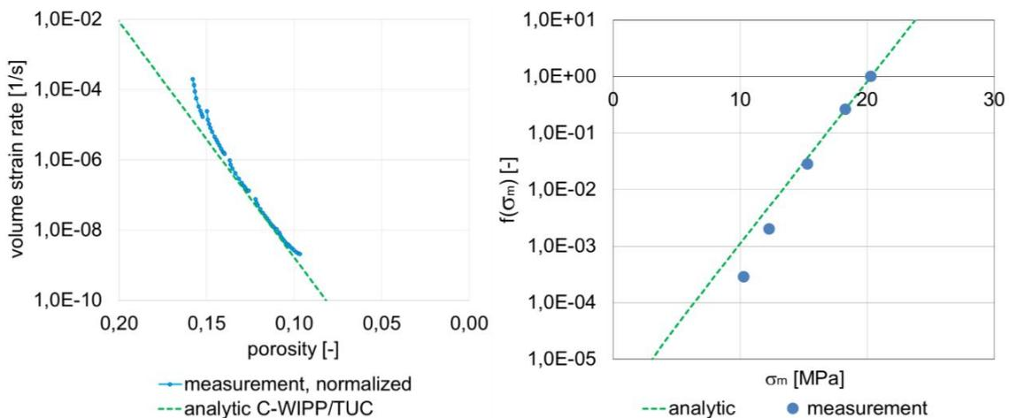
**Fig. 5.53** Parameter determination for the model C-WIPP/TUC using the experiment TK-031
