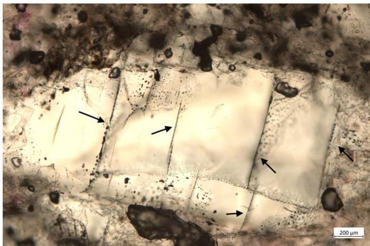
**Fig. 4.46** Sample 681/Oed1 a& b) Low magnification photomicrographs to observe pore structure and grain shapes and sizes, c) Crack propagating through grain in reflected light, d) Same location as image c, in transmitted light, to observe fluid inclusions near crack, e& f) Fluid inclusions in propagated micro-cracks (arrows) in transmitted light
