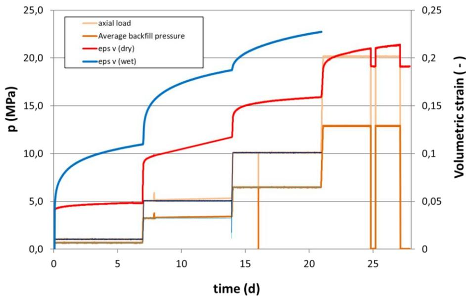
**Fig. 4.33** Multistep load tests in the “Big compaction cell” with different initial water contents (0 – red curve - and 1.0 wt.-% - blue curve): volume strain and axial load respectively average backfill pressure vs. time
