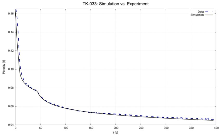
**Fig. 5.38** Simulated porosity evolution vs data for TK-033
