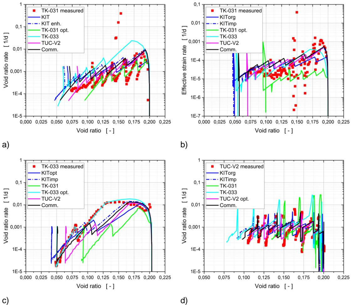
**Fig. 5.27** Measured and calculated deformation behaviour; calculation with all sets of parameters: a) Rate of void ratio of TK-031; b) Rate of effective strain of TK-031; c) Rate of void ratio of TK-033; d) Rate of void ratio of TUC-V2
