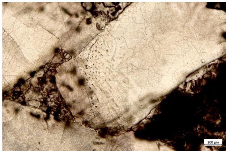
**Fig. 4.49** Big oedometer sample a) Impinged grain at center experiencing cataclastic deformation, b) Microcracks through grain, with transgranular crack at centre (red circle), c) Microcracks (arrows) through grains in transmitted light, d) Mechanically abraded surface between grains, e) Large crack propagating through grain (center right going left), f) Polygonal subgrain structure ranging in sizes from 50  $\mu\text{m}$  to 250  $\mu\text{m}$
