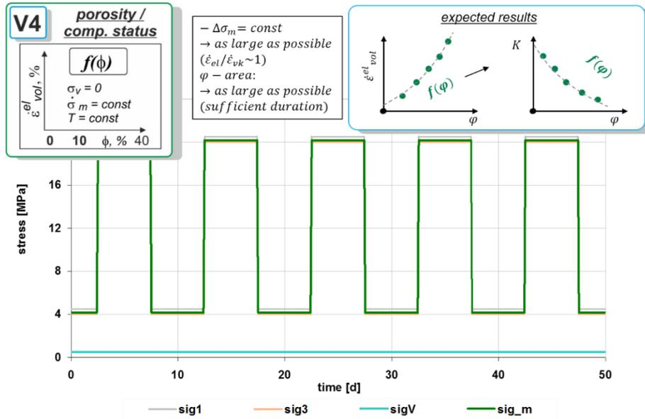
Fig. 6.11 Loading history of test type V4
