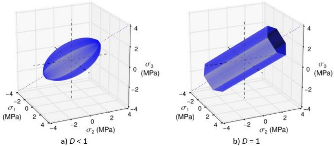
**Fig. 5.7** Flow potential at two different relative densities
