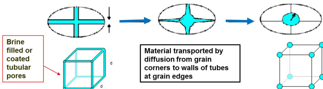
**Fig. 3.9** Schematic of fluid redistribution in granular aggregates during compaction. (left) initial situation with cubic grains and pore fluid channels along cube edges; (right) isolated spheres at cube corners
