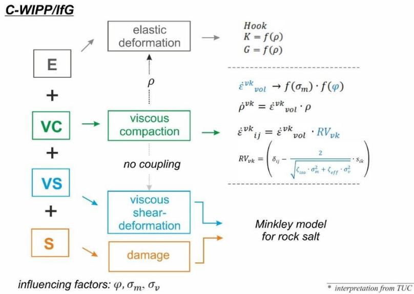
Fig. 5.17 Structural sketch for the constitutive model C-WIPP/IfG
