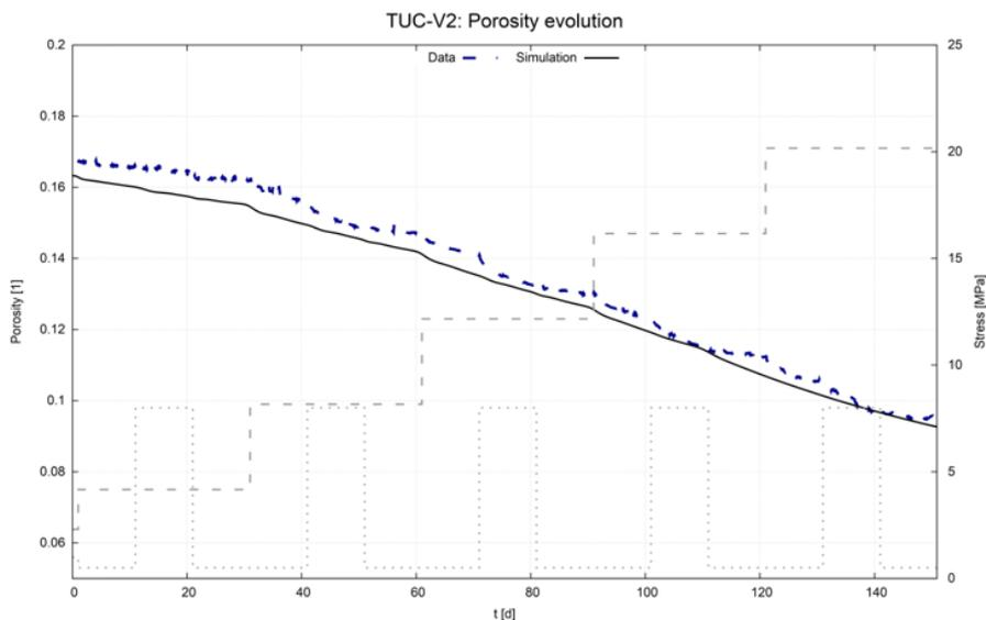
**Fig. 5.39** Simulated porosity evolution vs. data for TUC-V2
