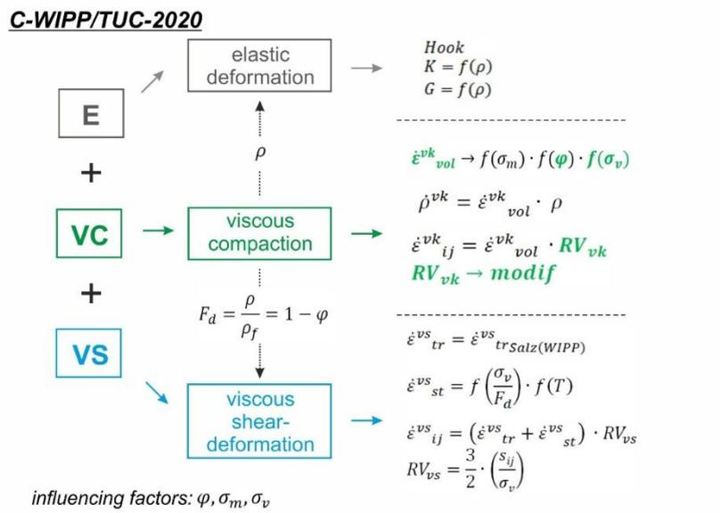
Fig. 5.18 Structural sketch for the constitutive model C-WIPP/TUC
