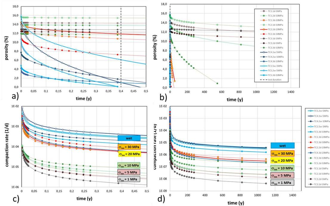
**Fig. 4.43** Calculated compaction and compaction rate curves, based on the experimental parameter sets given in Tab. 4.10: a) and c) for the experimentally investigated test duration; b) and d) extrapolated for a time scale > 1,000 years
