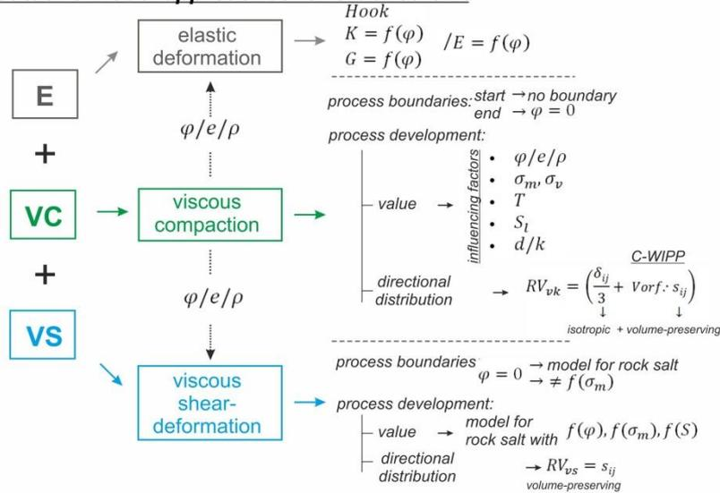
**Fig. 6.23** Formalized collection structure of the constitutive models for crushed salt: common features of the constitutive models, common need for validation and need for experimental investigations
