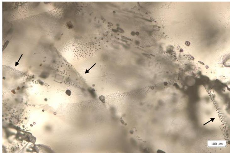
**Fig. 4.48** Sample 681/Oed3 a) Low magnification photomicrograph to observe pore structure as well as grain boundary diffusional pressure mechanism, b) Plastically-coupled pressure solution grain deformation at centre (Grain 2). c& d) Fluid inclusions in propagated micro-cracks (arrows) in transmitted light
