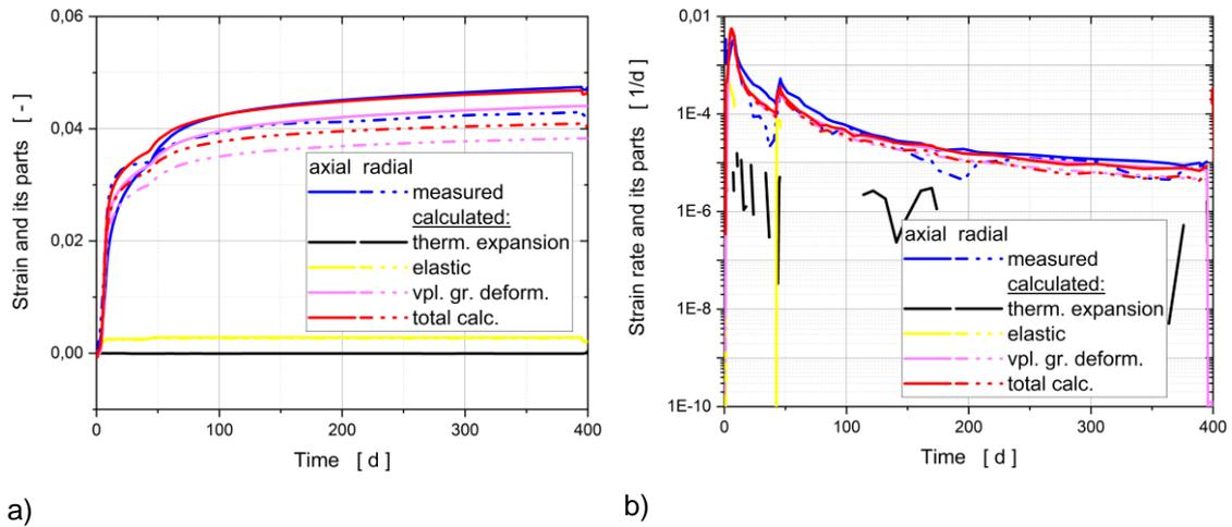
**Fig. 5.26** Measured and calculated deformation behaviour of TK-033, calculation with parameter set TK-033: a) Components of strain in axial and radial direction, b) Components of strain rate in axial and radial direction
