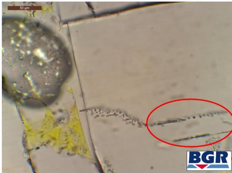
**Fig. 4.54** Fluid inclusion lines (red circle) in compacted crushed salt, scale bar is 50  $\mu\text{m}$
