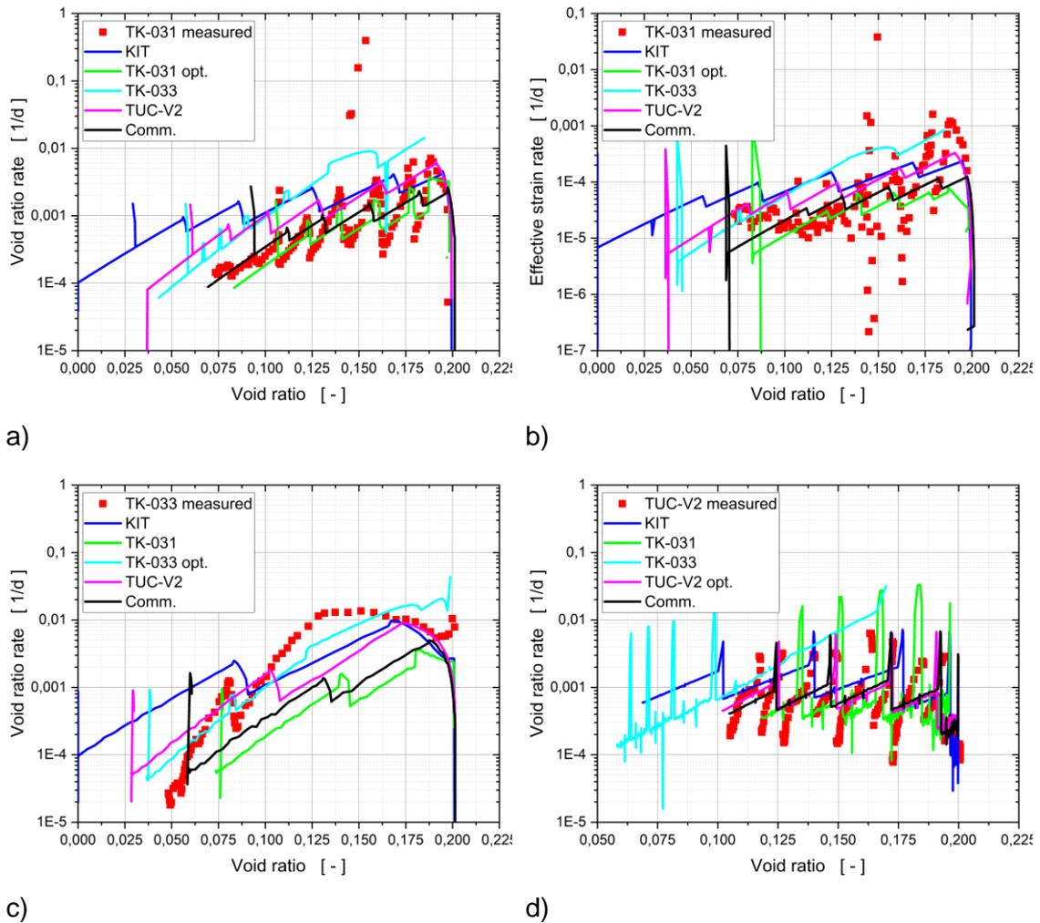
**Fig. 5.25** Measured and calculated deformation behaviour; calculation with all sets of parameters: a) Rate of void ratio of TK-031. b) Rate of effective strain of TK-031. c) Rate of void ratio of TK-033. d.) Rate of void ratio of TUC-V2.
