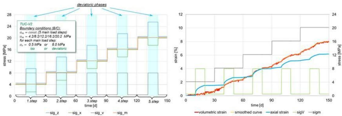
**Fig. 5.23** The load history and measurement results for the multi-stage long-term test TUC-V2
