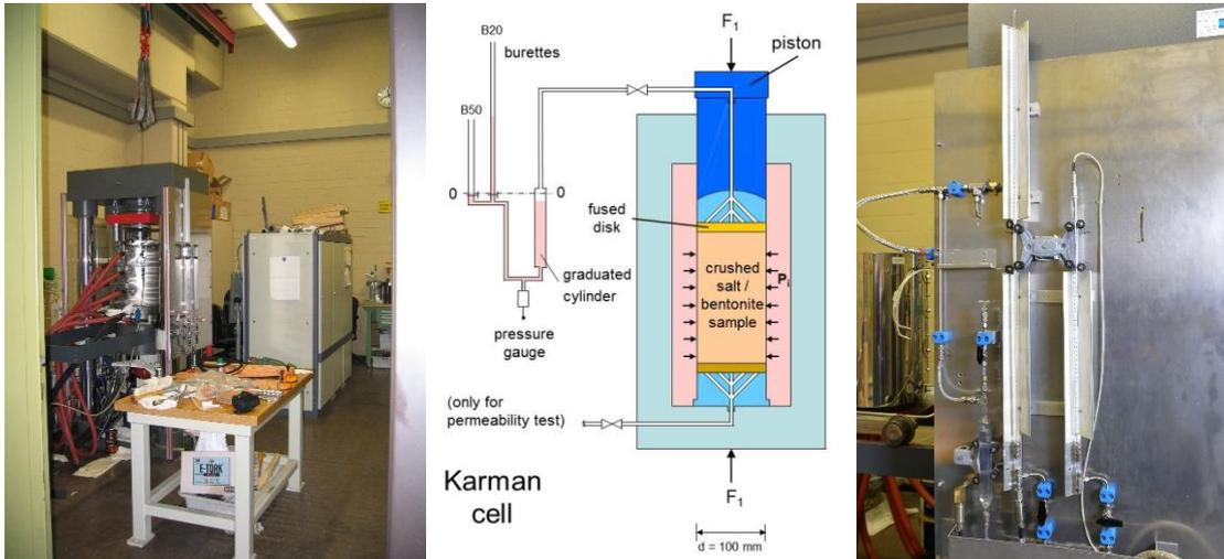
**Fig. 4.36** Triaxial testing system with load frame, sketch of the pressure cell and the burette system
