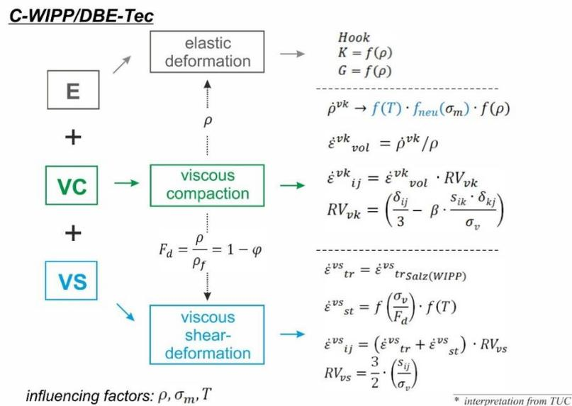
Fig. 5.16 Structural sketch for the constitutive model C-WIPP/DBE-Tec
