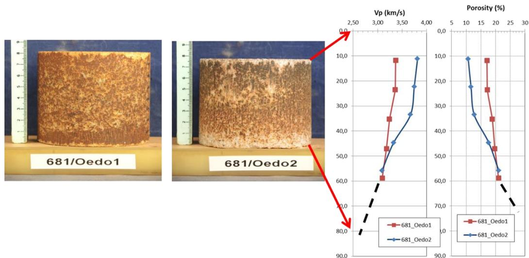
**Fig. 4.30** Pre-test specimens – test of homogeneity: (left) deformed specimens at 94 °C; (right) Ultrasonic wave velocity across the sample axis (radial measuring direction) at different heights and the resulting porosity
