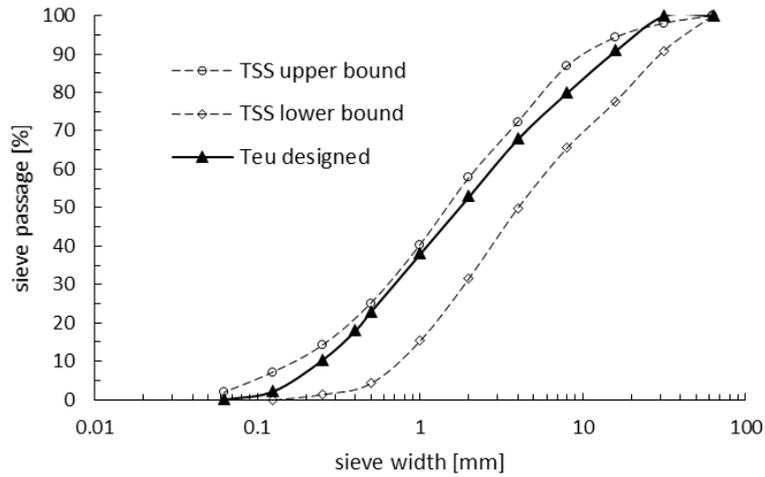
**Fig. 4.10** Grain size distribution curves. Solid line = designed crushed salt from Teutschenthal material, dashed lines = upper and lower bound of grain size distributions from crushed Asse salt as used in previous “TSS-tests” of the BAMBUS project
