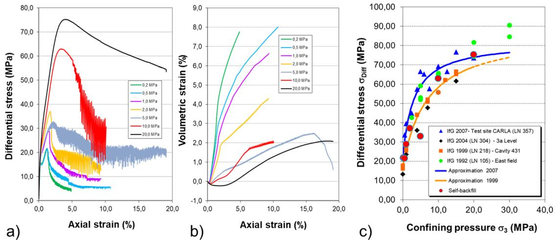
**Fig. 3.6** Summary of triaxial strength test on re-compacted self-backfill samples at 23 °C.
