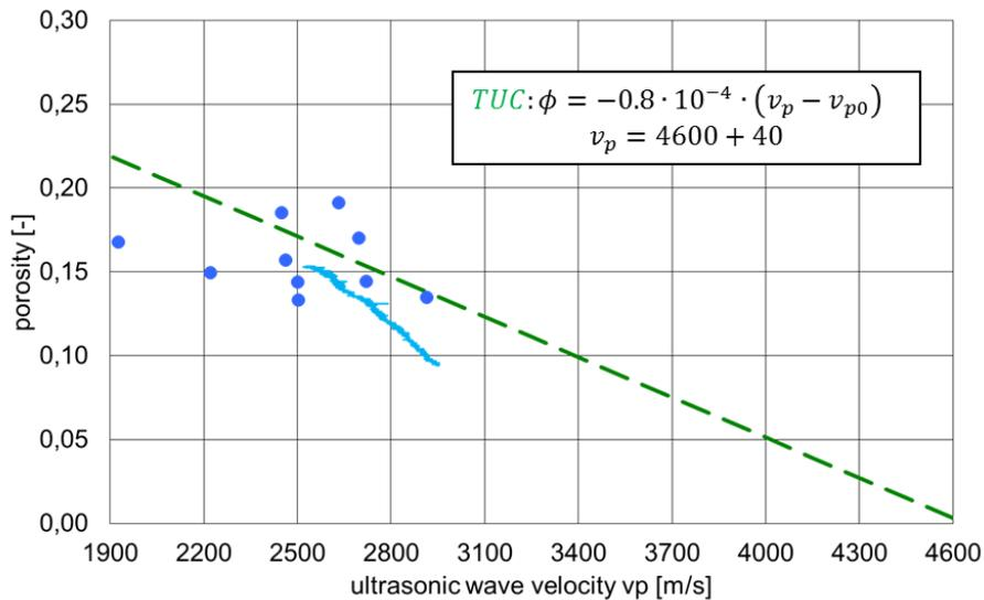
**Fig. 4.63** Course of the ultrasonic wave velocity in the TUC-V2 experiment in comparison to load-free measurements on pre-compacted crushed salt test specimens and the theoretical functional dependence
