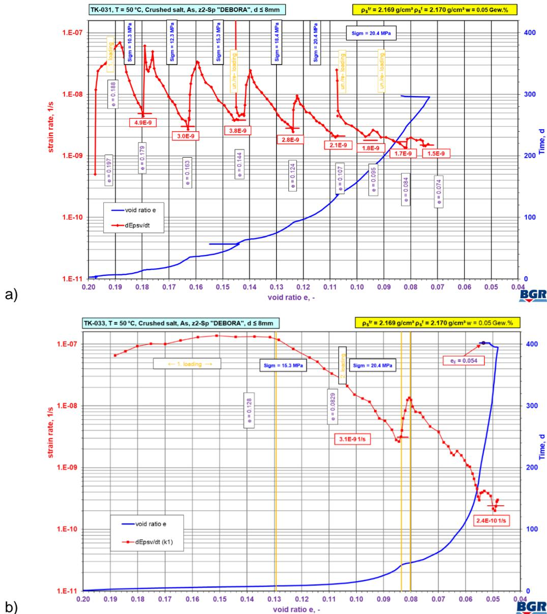
Fig. 4.40 Development of strain rate versus void ratio for a) TK-031 and b) TK-033
