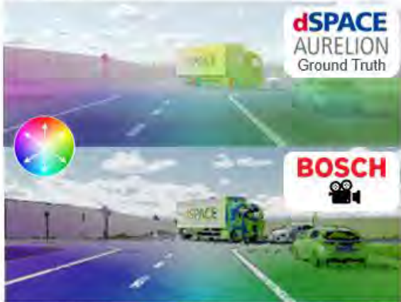
Image 1: (dSPACE visualization) Optical flow shown as an overlay, derived from ground truth data. Velocity and direction are encoded in HSV color space.
