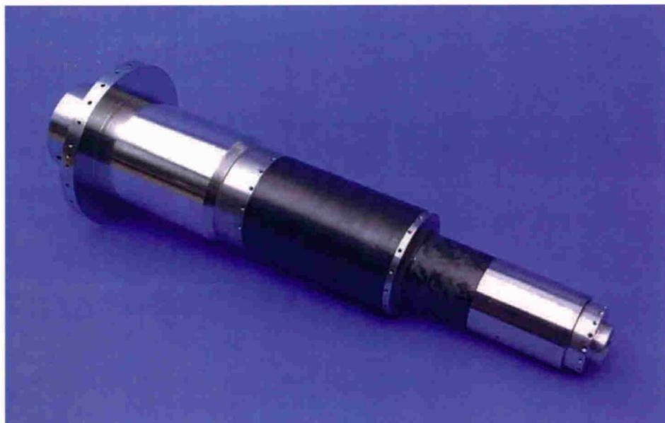
**Figure 9: Finished carbon fibre spindle rotor**
