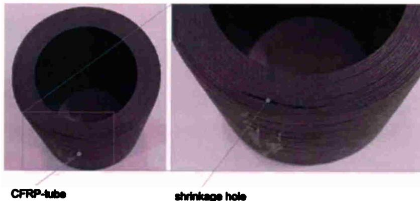
**Figure 6: Shrinkage holes within the CFRP-tube**
