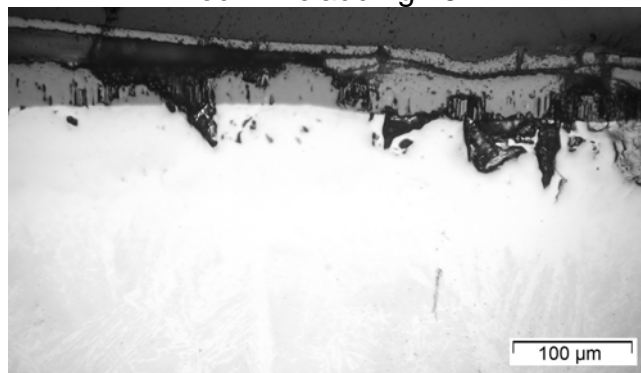
Rod 21, 45°: external oxide scale spalling
