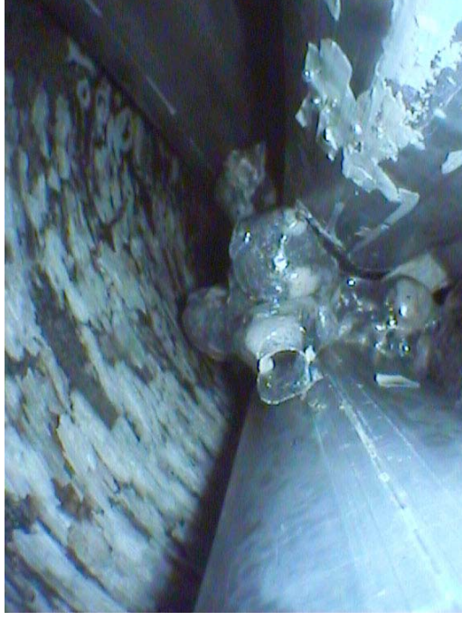
Melt formation in bundle at the break position of the corner rod
