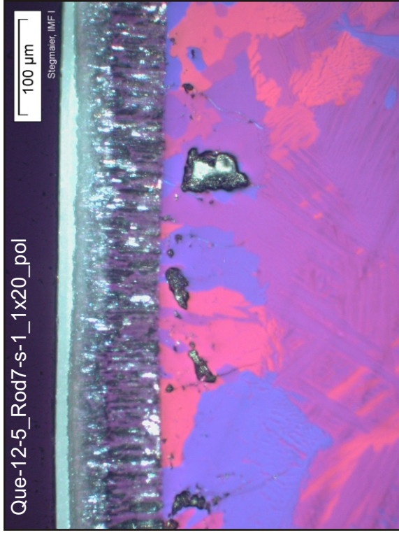
Fig. 71: QUE-12-5, level 750 mm; cladding oxidation of rods 2 and 7 (inner ring, heated).
