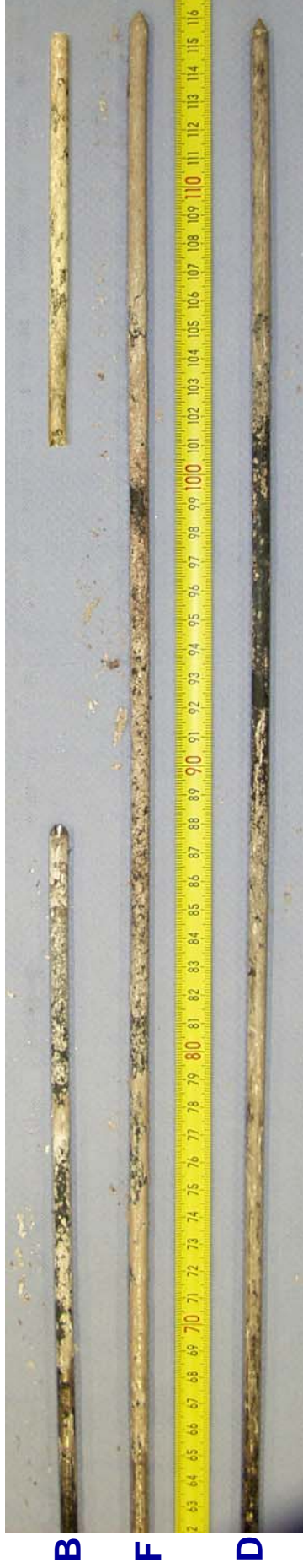
Corner rods withdrawn during the main test : D – after pre-oxidation, F – before reflow, B – after test.
