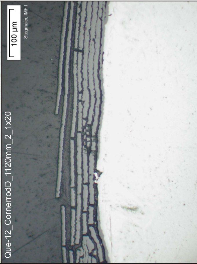
Fig. 118: QUE-12, level 1120 mm; oxidation of withdrawn corner rod D, representing the end of the pre-oxidation phase.
