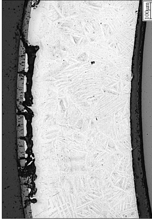
Fig. 147: QUENCH-12; Structure of the simulator claddings in cross section 654 mm (simulator 6 heated, simulator 10 unheated).
