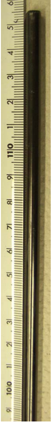
corner rod B after pre-test (800 °C, oxide layer thickness < 5 µm, measured with eddy-current technique)
