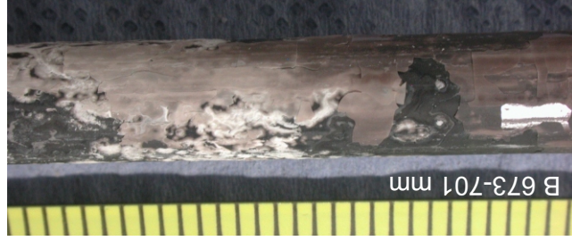
Fig. 122: QUE-12, level 700 mm; oxidation of withdrawn corner rod B, representing the whole test exposure.
