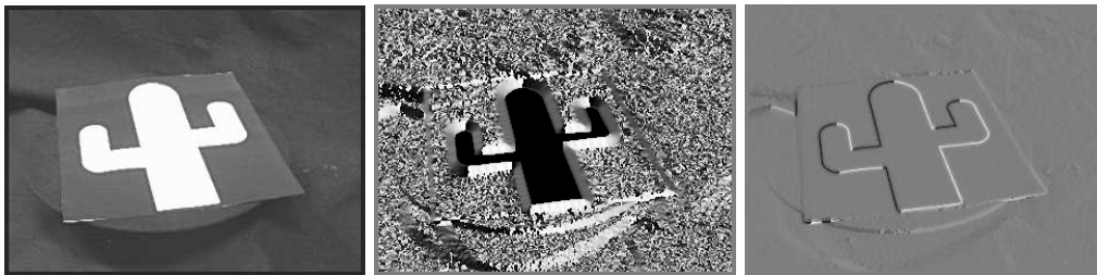
Fig. 4.7: Example of the monogenic signal response of an image. Original image (left), local orientation (center) and phase (right).
