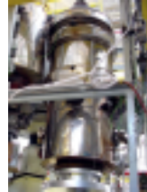
CUTEc fluidized bed reactor (150 kW)
