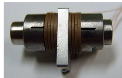
Fig. 4: Prototype of the bending type Langevin transducer
